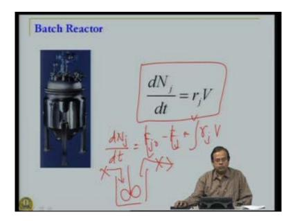
So going back our mass balance general mass balance equation is this. Let us consider a batch reactor. In a batch reactor we know that there is no in flow, there is no out flow that is why both these terms disappear and stirred time reactor operated in the batch mode. So conditions are uniform throughout the entire reactor and we have dN j dt as r j into V as our mole balance straight forward exercise.
