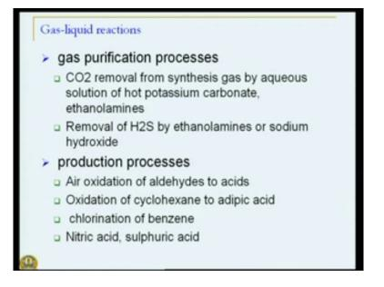
We have things like carbon dioxide removal from synthesis gas for example, using aqueous solution of hot ammonia, a hot potassium carbonate or ethanolamines. So, C O 2 removal, essentially it could be in the synthesis gas or it could be in the thermal power plant flue gases from thermal or whichever may be the case. The idea is that you want to remove it in hot potassium carbonate or ethanolamine.
