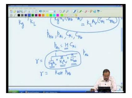
So, this one for example, this one for example, this whole thing is under, this one for example, tells us that this is now my equivalent rate constant, which is not essentially same as the kinetic rate constant. But this is how. So, let us say we can say this as k effective into partial pressure of A B that is my rate.
