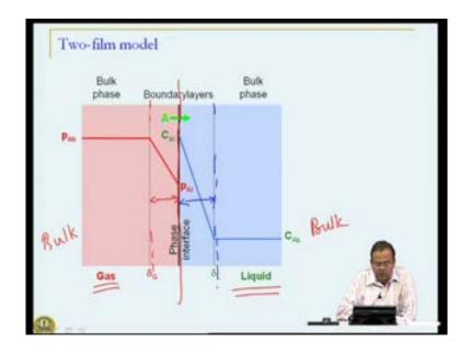
But let us look at the broad framework under which these reactions are often looked at. And this broad framework is that of a two-film model. So, what we have here is, let us say that we have a reaction between a and b, but even before we come to the reaction of a and b that is, a is a gaseous component, b is a liquid component. Let us try to look at what will happen when gas and liquid are brought in contact with each other. And that forms the basis of two-film theory.
