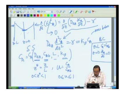
So that, we before we move onto looking at the actual results. What we have here, is dow dow t of epsilon concentration is dow dow Z of D e A dow C A dow Z minus r. The first simplification, that we are and this is we are describing a slab Z equal to 0, Z equal to 1 diffusion and reaction over here.
