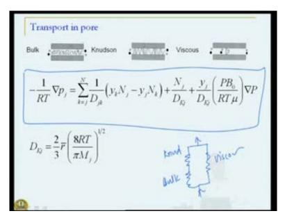
And hence this term which involves pressure drop driven. What you see here what you see here as a model of entire diffusion is what is referred to as mason Andean's dusty gas model, which assumed Knudsen and bulk diffusion in series. So, the actual model used is analogy with an electrical circuit.
