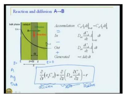
So, now having got some idea about how the material is moving through this catalyst pellet. Let us now turn our attention, actually to reaction and diffusion. What we are now going to do is look at a mass balance, which is applicable when material is both diffusing and reacting.
