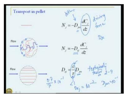
This is not the end of the story, because as you can see here we have represented this catalyst as a single pore. But catalyst, of course is not a single pore. It is a pore, catalyst actually is a combination of different sizes of pores, different orientations of pores and so on.
