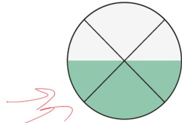
**Figure;** Shadow boundary of total reflection in an Abbe refractometer
