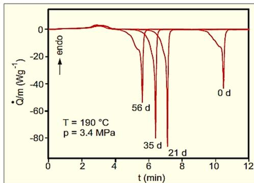
✓ Figure shows the impact of oven ageing on the oxidative induction time, which was determined using POM homopolymer pellets at 190 °C and 3.4 MPa of pressure.
