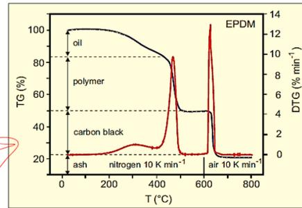
Thermal degradation behavior of EPDM
