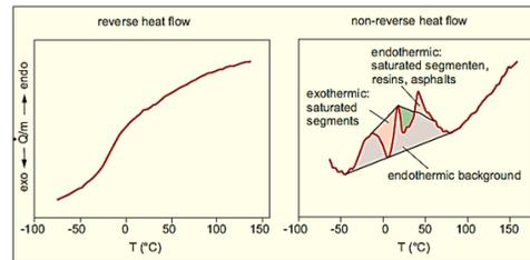
Use of temperature modulated DSC (TMDSC) for characterizing bitumen
