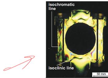
**Figure;** showing Stress optical image of model body under loading in linear polarized transillumination
