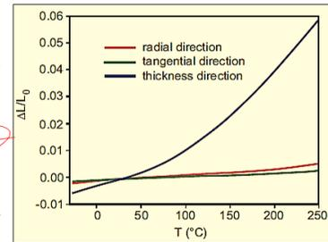
**Figure;** Showing thermal expansion of a fiber-reinforced PPS plate
