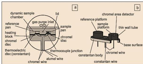
**Fig. (a)** Structure of a DSC measuring cell (heat-flow principle) disk tester system **(b)** structure of a Tzero™ sensor (TA Instruments)
