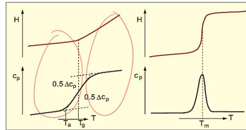
**Figure;** Showing glass transition with  $T_g$  determination and melting range
