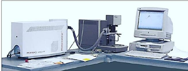
Thermogravimetric analysis coupled with a quadrupole mass spectrometer
