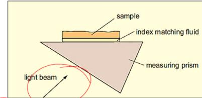
Arrangement of refractive index determination on solid materials using a refractometer.
