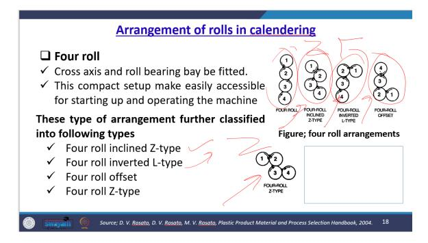
In the inverted L type configuration, the arrangement resembles an inverted "L" shape, as illustrated. The Z type features four rolls in a Z-shaped configuration, offering a specific setup for calendaring operations. The four-roll offset design is characterized by an offset arrangement, contributing to the machine's overall efficiency.
