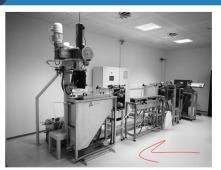
Figure; Synthetic fiber spinning machine
