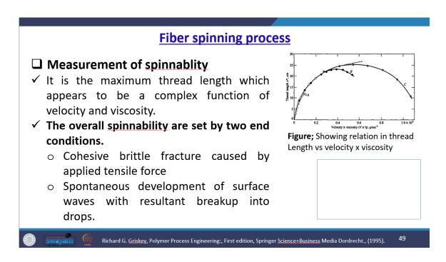
In summary, the overall spinnability of synthetic fibers is influenced by two key end conditions: cohesive brittle fracture caused by applied tensile force and the spontaneous development of surface waves leading to breakup into drops. These conditions highlight the delicate balance required in the spinning process to avoid undesirable outcomes and achieve successful fiber production.
