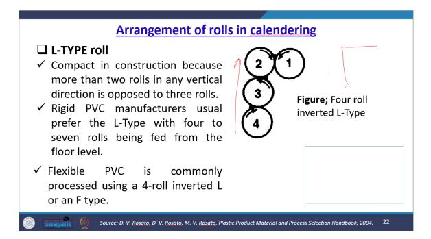
The universal five-roll L calendar finds application in processing both rigid and flexible PVC films. This configuration offers heat stability, superior film control, and a desirable surface appearance. Notably, this system has the capability to allow plasticizer-saturated vapors to escape through the suction hood located above the calendar, passing through filters before being released into the atmosphere.
