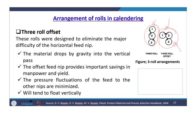
The pressure fluctuations from the feed to the other nips are minimized in configurations designed for vertical floating. In the realm of four-roll setups, various combinations exist, such as the four-roll incline Z type, L type, and four-roll offset. These configurations may incorporate cross-axis adjustments and roll bearings, ensuring a compact setup that is easily accessible for machine startup and operation.
