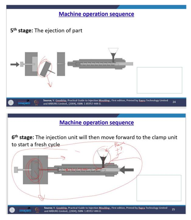
The injection molding cycle this can be broken down into 3 distinct stages one is plastication, second one is the mold filling and third one is the cooling with
