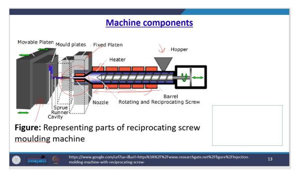
Now this injects the molten material to a closed mold. Here you see that this is the closed mold. There are various channels through which it can go inside the mold with the gates and runners. Then it cools the mold because it is a heat and plasticized material. So obviously you need to cool the mold otherwise once you remove the part then definitely it may deform over the shape.
