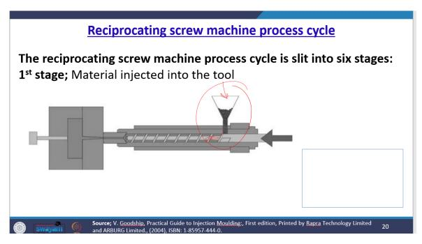
So, the second stage this screw begins to turn and retract the metering a specified weight of molten material for the next shot and the previous shot which is being inserted is now cooling and in the closed tool. So, this can be come out. The third stage the injection molding unit moves back from the clamping unit. So, this movement is like this. So, the machine is preparing itself for the next shot.
