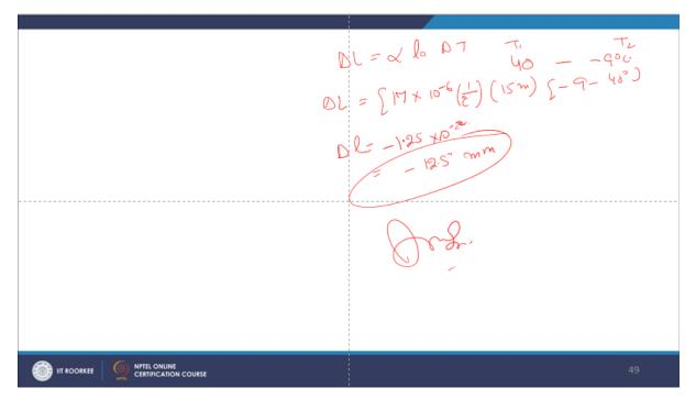
So minus 9 to 40 degree Celsius. So delta L comes out to be minus 1.25 into 10 to the power then it is comes out to be minus 12.5 mm this is the answer. Let us talk about the thermal stress. This stress due to the change in temperature or due to temperature gradient this is termed as a thermal stress.
