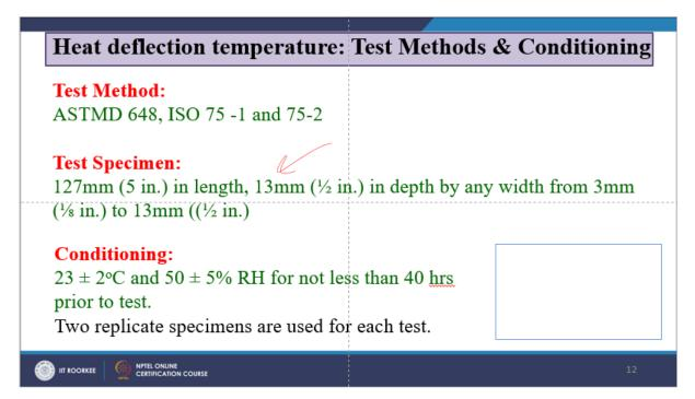
So, the condition requires a specified temperature and relative humidity. So, this is 23 plus minus 2 degrees Celsius and 50 plus minus 5 percent of relative humidity not less than 40 hours prior to the test. Now, two replicate specimens are used for each test so that the efficacy of the experiment can be evaluated. Now, this is the apparatus where you can have you can determine the HDT. Now usually
