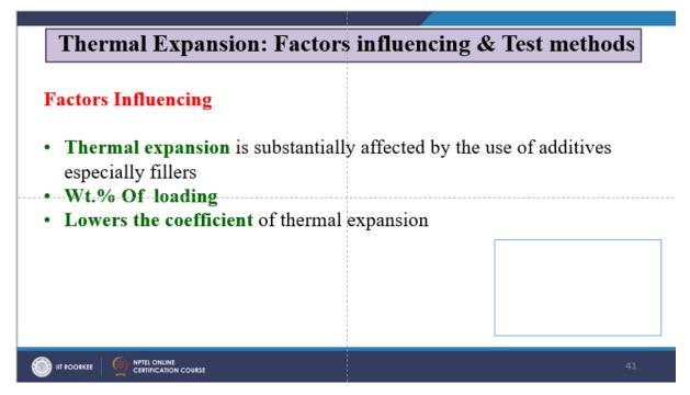
The factor influencing the thermal expansion is substantially affected by the use of additives especially fillers because during the processing of the polymeric product you need to add certain additives, fillers, dyes, chemicals all these things and these play a very vital role.
