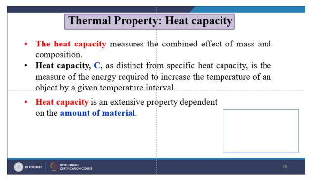
This is distinct from the specific heat capacity. This is measured by the energy required to increase the temperature of an object by a given temperature interval. Now, heat capacity is an extensive property depending on the amount of material. Now, let us talk about the atomic vibration. The atoms and ions that are bonded together with considerable inter-atomic forces are not motionless. Due to the consistent vibration movement they are permanently deviating from their equilibrium position.
