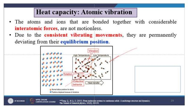
Now, here you see that these are the molecules in some of the rotations and collective behaviors. Now, atomic vibrations are in the form of lattice waves or phonons. Now, faster molecules shrink slower ones, the boundary in the elastic collision will increase the velocity of the slower ones and decrease the velocity of the faster ones. Transfer sometimes they need to transfer the energy from the higher temperature to the lower temperature region.
