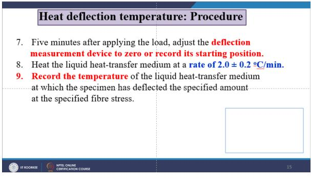
Now, heat the liquid heat transfer medium at a rate of say 2.0 plus minus 0.2 degrees Celsius per minute. You need to record the temperature for the liquid heat transfer medium at which the specimen is deflected by a specified amount at the specified fiber stress. Now, how can we calculate it? The weight of the rod used to transfer the force on the test specimen is included as a part of the total load.
