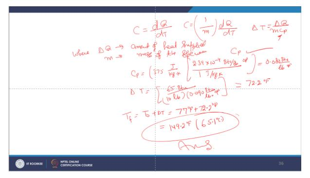
Now this CP is given to you. Now this where delta Q is the amount of heat supplied and m is the mass of the specimen and CP is always given to you. So CP is equal to 375 joule per kilogram Kelvin 2.39 into 10 to the power minus 4 BTU upon and this comes out to be 0.080 BTU. Now delta t is equal to 65 BTU which is given in the problem and 10 pound into 0.
