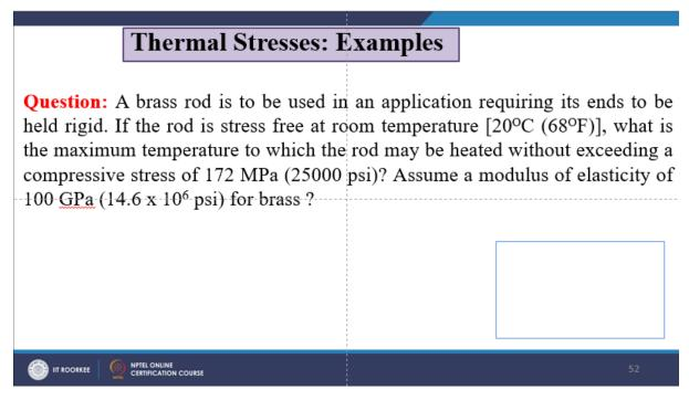
Then another is assuming unconstrained thermal expansion where this having a delta L length change this is original L naught from here to here and this is delta L. Now here delta L over L at room is equal to and which is represented as alpha L T f minus T naught final temperature minus T naught this is at the final temperature. Now another step the compress specimen back to original length. So, small sigma which is L naught and you see that this is the delta L which need to be compressed.
