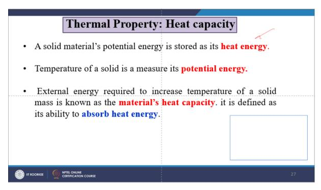
So, this particular thing is extremely important. Now let us talk about the heat capacity. Solid material's potential energy is stored in heat energy and the temperature of the solid is measured as its potential energy. So, the external energy required to increase the temperature of the solid mass is known as the material heat capacity and it is defined as its ability to absorb heat energy. So, the heat capacity measures the combined effect of mass and composition and usually it is denoted as C.
