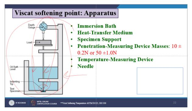
Now this is the softening point apparatus. Here you see that there is an immersion bath and usually when we have the heat transfer media then the specimen support and penetration measuring device masses and the temperature measuring device and there are needles.
