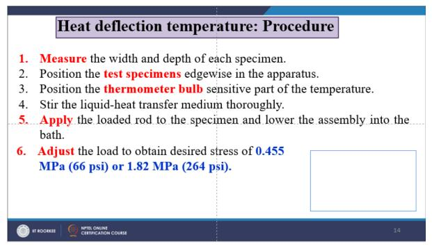
For this you need to calculate the depth gauge. Now adjust the load to obtain the desired stress of say 0.455 mega Pascal or 1.82 mega Pascal. So, you need to wait for 5 minutes after applying the load and then deflection the measurement device to 0 or record its starting position.
