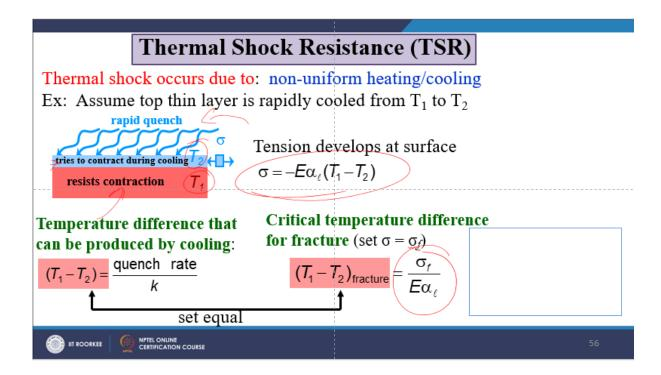
$$(T_1 - T_2)_{\text{fracture}} = \frac{\sigma_f}{E\alpha_\ell}, \quad (T_1 - T_2) = \frac{\text{quench rate}}{k}$$
