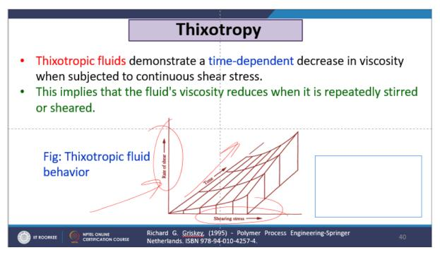
These fluids can be thought of as a fluid in which tau is equal to phi d gamma over dt t. This is the thixotropic fluid behaviour where nita is the initial viscosity and infinity is the viscosity after infinite time. So, this is the generalized rate of shear versus apparent viscosity. Now, let us talk about the yield stress and time dependent behaviour. The yield stress, these fluids have a threshold stress known as
