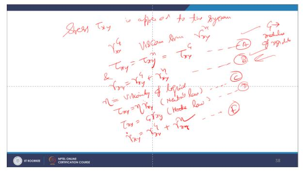
So, tau xy gamma xy bar that is Newton's law and tau xy is equal to g xy that is Hooke's law. And g is the modulus of rigidity. So, if we differentiate this equation that is equation number B, it becomes is equal to. So, if we combine equation A, B and E with equations C and D, so it becomes d tau xy dt is equal to g gamma xy dt minus tau xy lambda, where lambda is equal to g over.
