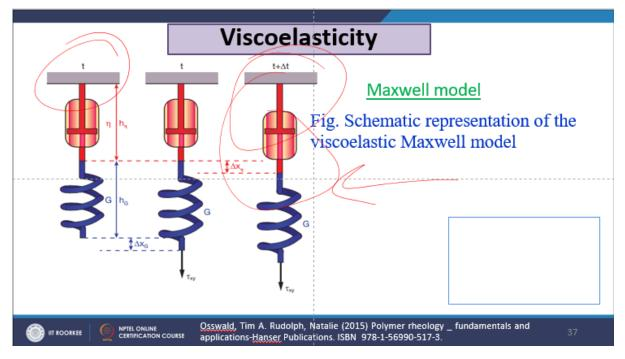
Total strain is the sum of elastic strain that is gamma xyg and the viscous strain xyn. So, tau xy is equal to tau xy n is equal to tau xy g. This is let us say equation A and gamma xy is equal to gamma xy g plus gamma xy n. This is let us say equation number B. Now, if we take this, this is the viscosity of liquid.
