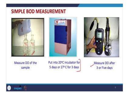
Now, these are the bottles we can see the initial these are the 300 ml bottle, they essentially when we fill the water in this water bottle sample in this water bottle actually they when the cap is kept, they measure 300 ml exactly. So, we keep these bottles inside this incubator depending upon the temperature for that respective number of days and we measure the DO using the DO meter either 3 days or 5 days, we can use the titration method also for determining the dissolved oxygen.
