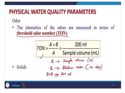
The intensities of the odors are measured in terms of threshold odor number (TON).
