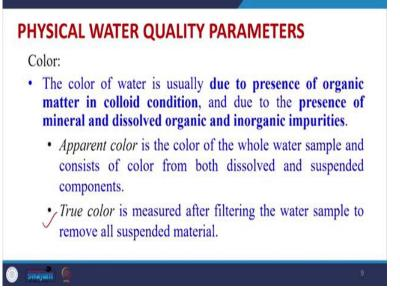
Then in the physical water quality parameter color is also an important parameter and color is also important for biological treatment of water also in particular if the water is generated in industry like textile and we are performing some water biological treatment process so we have to measure the color removal efficiency etcetera also. So color measurement is very important and color removal efficiency measurement is for most important for treatment process.
