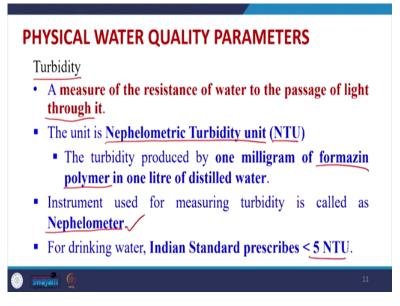
So turbidity actually measures the resistance of water to the passage of light through it. So we have how much light is absorb while the light is passing through the water samples that is given by the turbidity. Now this turbidity is measured in terms of unit which is called NTU, NTU means nephelometric turbidity unit and that turbidity as 1 NTU is the amount of unit which is actually produced by 1 milligram of formazin polymer in 1 liter of distilled water.
