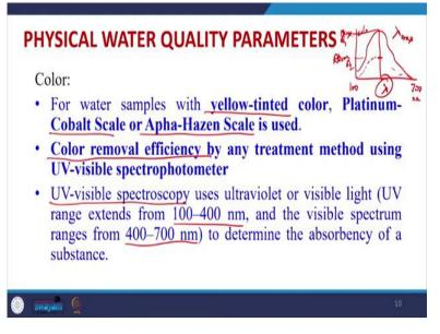
For water samples with yellow tinted color there is a method which is used for reporting the color of the water. So if any water which is yellow tinted remember it is for yellow tinted color. So the platinum cobalt scale is used and it is also called Apha-Hazen scale. So remember it was given by Hazen and it is used for reporting color of the water samples with yellow tinted color. So this and the instrument is also available for this.
