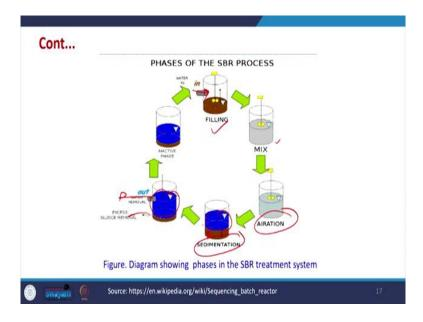
Then we have a mixing process where mixing is done. So, in this case the water is coming in. So, this is there, then we have mixing after that the aeration is being done and then the sedimentation after treatment of sedimentation, the sludge is here the blackish one, the and then the brownish one and the blue is the wastewater and the wastewater treatment has happened that is why it has become blue.
