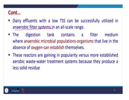
Dairy effluents with low TSS can be successfully utilized in the anaerobic filter system in all scale range. So, we can use the anaerobic filter also. The digestion tank contains a filter medium where anaerobic microbial population organisms live in absence of oxygen. Now, these reactors are gaining in popularity versus more established anaerobic wastewater treatment system because they produce less solid residue. So, this is there.
