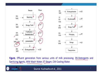
Now, the effluent generation from various units of the milk processing. So, here like DS stands for detergents and sanitizing agents. So, we use processes which are there receiving the water then storing it in the tank, then clarification and standardization, then pasteurization homogenization, after that deodorization, again storage, packaging, further storage and transportation.
