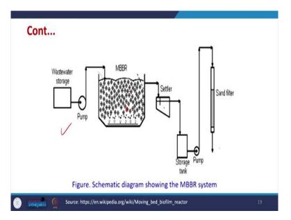
And we can see here the wastewater storage, this is activated sludge process in a way where on the packing material different bacteria have grown and the treatment will happen here and then the wastewater will be settled and it the sludge will be reduced and then the wastewater can be stored and further may be filtered through the sand filter. So, this is the treatment method via MBBR technique for daily wastewater treatment.
