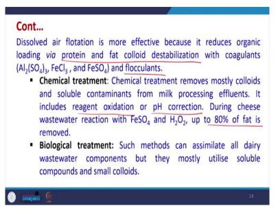
Dissolved air flotation is the most effective because it reduces the organic loading via protein and fat colloid destabilization with coagulants such as coagulants, such as aluminium sulfate, ferric chloride, ferrous sulfate, and the flocculants as well. Then we can go for chemical treatment which removes mostly collides and soluble contaminants from milk processing effluence.
