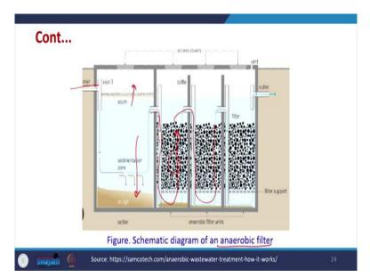
Now, this is the schematic diagram of anaerobic filter. So, here you can see the inlet is there and here some sedimentation is happening, the scum is going up and here the sludge is
