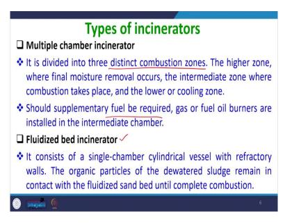
So, the first is the multiple chamber incinerator. In this incinerator, it is divided into three distinct combustion zones. The higher zone where the final moisture removal occurs. The intermediate zone where the combustion takes place and the lower or the cooling zone. It requires supplementary fuel gas or fuel oil burners have to be installed in the intermediate chamber where the combustion takes place.
