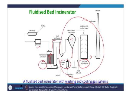
So, this is the fluidized bed reactor, schematic of fluidized bed reactor with washing as well as cooling gas systems, so both are there. So, this is the overall schematic diagram. So, this is the main furnace we can see here and after that this section you can consider as the air pollution or heat exchange area. So, we have sludge which is centrifuge and then we have pre-dire, it goes into the combustion chamber where fuel oil is there and air is there.
