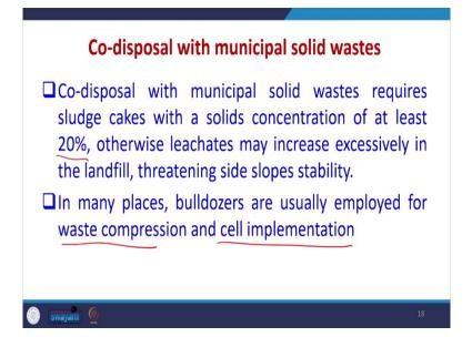
If we are going for co-disposal with municipal solid waste, then it will require sludge cakes with solid concentration of at least 20 percent, otherwise leachates may increase exclusively in the landfill, threatening side slopes stability as well as leaching going into the water.
