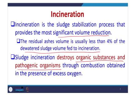
So, inspiration we are going to study today. Incineration is the sludge stabilization process that provides the most significant volume detection. So, during incineration we have the highest amount of volume reduction taking place and we get energy as well.
