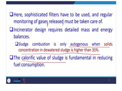
Here, but we have to take care of certain aspects, sophisticated filters have to be used and regular monitoring of gases released must be taken care of. So, we have to do the monitoring of the gases as well as we have to take care of that gases released if they are anything undesirable is happening. Incineration, their design requires detailed mass and energy balances.
