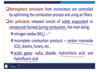
The atmospheric emissions from incinerators are controlled by optimizing the combustion process and using air filters. So, this is very important that we have this section which is like Air Pollution Control devices which are installed. So, you should control the emissions which are taking out of a combustion chamber. Air pollutants released consists of solids evaporated and compounds form during combustion.
