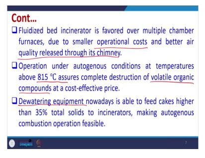
The fluidized bed incinerator is favoured over multiple chamber furnaces due to small operational cost and better air quality released through its chimney. So, generally the fluidized bed insulator will be preferred as compared to the multiple chamber incinerator and this is so, because the operation cost is also low and also the quality of air, the flue gas which are coming out are better as compared to the multiple chamber furnaces.
