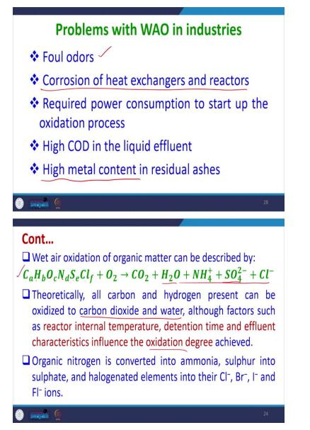
The problems with wet air oxidation in industries is, that we may have foul order. The corrosion of heat exchangers and reactors, because we have gases which are coming out as well as the halogenated materials which are coming out. So along with ammonia etcetera. So that may cause the problem. So this corrosion of heat exchangers and other reactors is the issue when we are using wet air oxidation and also of the wet air oxidation reactor itself the corrosion may happen.
