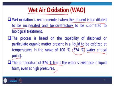
After thermal drying process there is another process which is called as wet air oxidation. So we can use the wet air oxidation technique also as one of the sludge transformation method. So wet air oxidation is recommended when the effluent is too diluted to be incinerated and toxic refracted to be submitted to the biological treatment.
