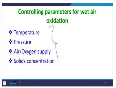
The parameters which may affect the wet air oxidation are temperature, pressure, air oblique oxygen supply, and the solid concentration which is there. So any all these four parameters may affect the wet air oxidation process in greater details.
