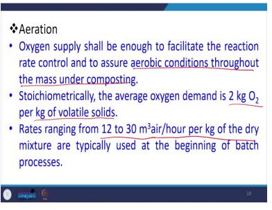
Now aeration because we this process is like aerobic process. So oxygen supply shall be enough to facilitate the reaction rate control and to assure the aerobic conditions throughout the mass under composting. So we have to see that oxygen is available for the aeration reaction, otherwise if oxygen is not available, we will not be able to properly do the composting.
