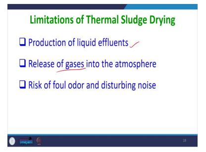
Now certainly there must be some limitations also of thermal sludge drying and these limitations are production of liquid effluence during the thermal sludge drying, release of gases also into the atmosphere depending upon the type of material which it contains, risk of foul odor and disturbing noise also occurring during thermal sludge drying.
