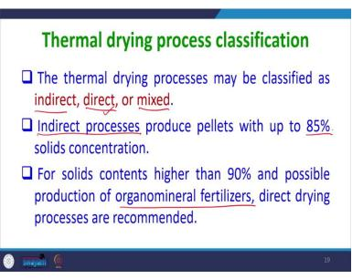
Now a thermal drying processes can be classified also. So there are three classifications of thermal drying processes, they are indirect, direct, or mixed. Now the indirect processes they produce pellets with up to 85 percent solid concentration. For solid contents higher than 90
