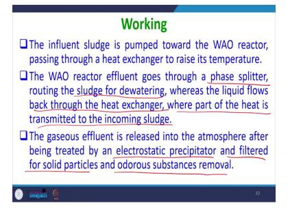
Now this is the working. The influent sludge is pumped towards the wet air oxidation reactor passing through the heat exchanger to raise its temperature. The wet air oxidation reactor effluent goes through a phase splitter, routing the sludge for dewatering, whereas the liquid flows back through the heat exchanger, where part of the heat is transmitted to the incoming sludge.
