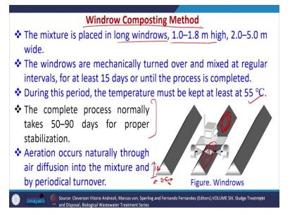
Now windrow composting method is one of the common most method which is used for composting, the in this case the mixture is placed in long windrows. So you can see the windrows which are there around 1.0 to 1.8 meter high, and then this is 1.8, and this is 2 to 5 meter wide. So it may vary from 2 to 5 meter. The windrows are mechanically turned over and mixed at regular intervals for at least 15 days.
