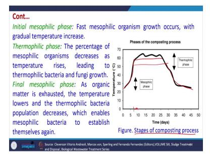
So there are certain stages in the treatment the there is initial mesophilic phase the fast mesophilic organisms growth occurs with gradual temperature increase. So you can see the mesophilic phase in which the temperature is increasing and it occurs between 7 to 10 days. So in this range the mesophilic phase will be there.
