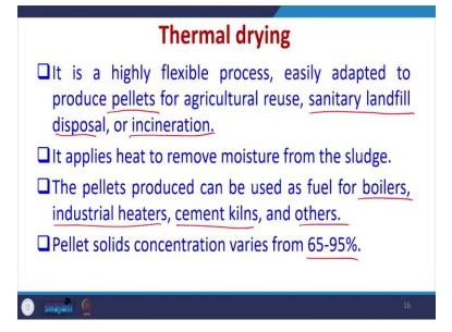
So let us start with thermal drying today. So thermal drying is a highly flexible process easily adapted to produce pellets of agricultural reuse, and sanitary landfill disposal, or incineration. So in this case it can be adopted to produce pellets. So we can produce pellets, we can finally dispose them off in the sanitary landfill or for incineration via thermal drying. So it applies heat to remove moisture from the sludge. So it is like sludge drying bed also.
