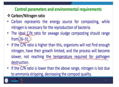
Now there are certain control parameters and environmental requirement. So one of the first important parameter is the carbon to nitrogen ratio. The carbon represents the energy source for composting, while nitrogen is necessary for reproduction of bacteria itself. So ideal C to N ratio for sewage sludge composting should range of 26 to 31.
