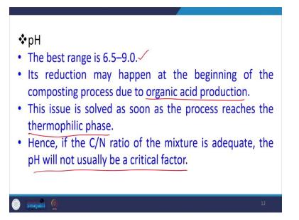
pH is also one of the important parameters for composting. So in this case the best pH range is 6.5 to 9. So if the pH is in between then the system works the composting occurs very well. If the pH reduces, its reduction may happen at the beginning of the composting process due to organic acid production which happens during the composting.
