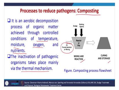
Now we can use the composting. So also, so composting is one of the method which is most commonly used. So it is an aerobic decomposition process of organic matter achieved through control conditions of temperature moisture oxygen and nutrients.
