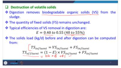
Typical efficiencies of VS removal in digestion are:
