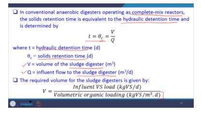
The solids retention time is equivalent to the hydraulic detention time and is determined by
