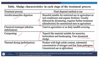
Now the sludge characteristics which will be obtained in each state of the thermal or this digestion process. So, we have aerobic or anaerobic digestion, we have chemical treatment, some chemical oxidation we can have composting, thermal drying etcetera.
