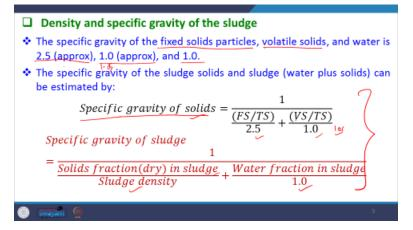
The specific gravity of the sludge solids and sludge (water plus solids) can be estimated by:
