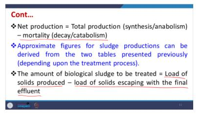
The net production will be or total production whatever via these two methods and then there is a endogenous respiration or catabolism happening or decay. So, that mortality among themselves the biomass that has to be subtracted. So, approximate figures for sludge productions can be derived using the tables which have been presented in the previous lecture.
