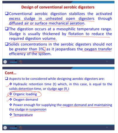
Now, let us consider the design also of conventional aerobic digester little bit. The conventional aerobic digestion stabilizes the activated excess sludge in unheated open digester through diffused air or surface mechanical aeration.
