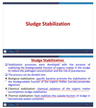
So, now we will go and try to understand the second step which is called as sludge stabilization. So, will be this is the B section.
