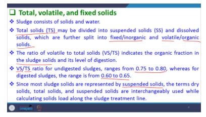
Since most sludge solids are represented by suspended solids the term dry solid, total solid, suspended solids are interchangeably used while calculating solid loads along the sludge treatment line. So, most of the data which is reported is based upon suspended solid. So, the dissolved solids content many times is missed and it means that dry solids, total solids, suspended solids they are used very interchangeably.
