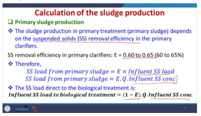
SS load from primary sludge =  $E \times Influent SS$  laad SS load from primary sludge = E.Q.Influent SS conc
