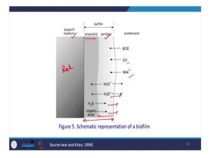
Now we can see here the schematic representation of biofilm we can see this is a support medium which may be rock also and then we have a biofilm which is there. So inside the biofilm there may be aerobic conditions in the first stages and after that there may be anaerobic condition depending upon the thickness of the film. So we have wastewater which is it is BOD, DO, NH<sub>4</sub> etcetera.
