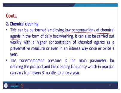
Then we have chemical cleaning, this can be performed by implying low concentration of chemical agents in the form of daily backwashing. So, that means, we have to daily back
