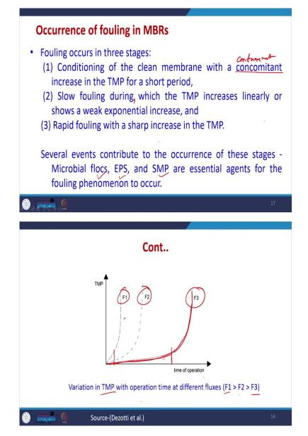
Now, Occurrence of fouling in the MBR. So, fouling occurs in a number of stages in particular like three stages. So, first that conditioning of the clean membrane with a contaminant increases in the TMP. This is contaminant increases in the TMP for short period. So, this is the first stage, then here the conditioning happens during the initial treatment itself.
