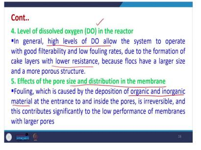
Also the level of dissolved oxygen in the reactor in general, the higher level of DO allow the system the biological system to operate with good filter ability and low fouling rates. So, that means, if we can maintain higher level of DO inside the biological reactor, the fouling in the module will be less due to the formation of cake layers with lower resistance and because flocs have a larger size and they will be blocked easily and the overall structure will be more porous.
