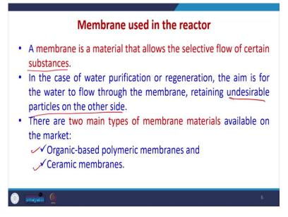
So, membranes used in the reactor which type of membrane has to be used, what material sector so, a membrane is a material that allows the selective flow of certain substance. So, this is the classic definition of membrane in the case of water purification our regeneration, the aim is for the water to flow through the membrane, but retained undesirable particles on the other side itself.
