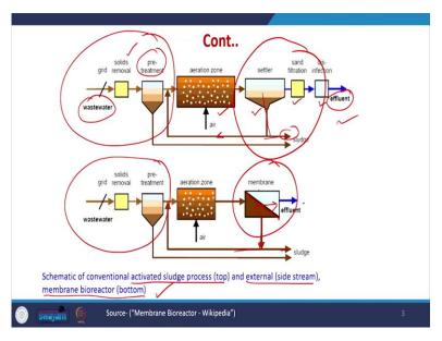
So, we can see here that traditional wastewater treatment using an activated sludge process. So, we have activated sludge process in which the wastewater is coming, the solid removal happening in the physicochemical treatment then some pretreatment happening after that, in the activated sludge, we have a air which is there and the treatment happening, after that we use the settler or the clarification unit where the settling happens some of the sludge is recycled back or other is wasted.
