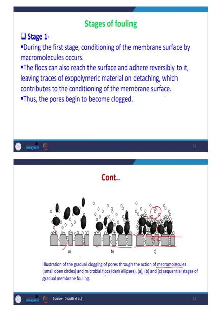
Now, we can see in the stage one during the first stage that conditioning of the membrane surface by macromolecules occur. So, we can see here the conditioning is happening and the floc s can also reach a surface and adhere reversibility to it, leaving traces of exopolymeric material and detaching which contributes to the conditioning of the membrane surface. Thus pores are becoming clogged here.
