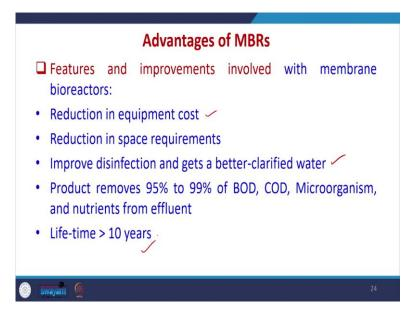
There are certain advantages of MBR. So, there are many features and improvements involved in the membrane bioreactors, one is the reduction in the equipment cost because we are not using the clarification system then also we do not need to use the sand filtration unit etc. So, we can have reduction in the equipment costs. Certainly the space requirement is much lower as compared to the activated sludge system followed by a clarification unit and a sand filtration unit.
