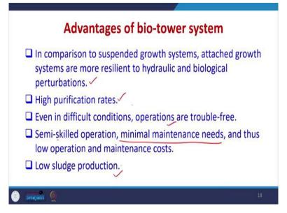
Advantages of bio towers in comparison to suspended growth system the attached growth systems are more resilient to hydraulic and biological perturbations, they have high purification rates, also in the difficult conditions operations are trouble-free.
