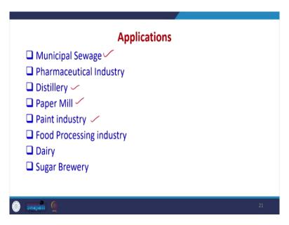
Now, these bio tower systems are used in many applications, they can be used for treatment of municipal sewage, they are recommended for treatment of like pharmaceutical industry wastewater, Distillery wastewater, paper mill, paint industry wastewater which contains very high organic loading, then food processing industry, dairy, sugar brewery etc.
