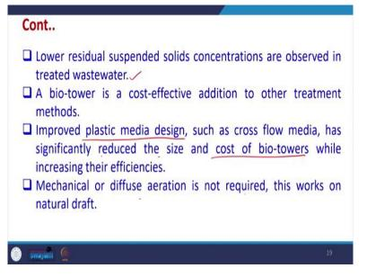
Now, the lower residual suspended solid concentrations are observed in the treated wastewater of such system, because some filtration also happens. A bio tower is cost-effective addition to the other treatment method as compared to other, but it efficiency may vary be depending upon the wastewater characteristics and other parameter.
