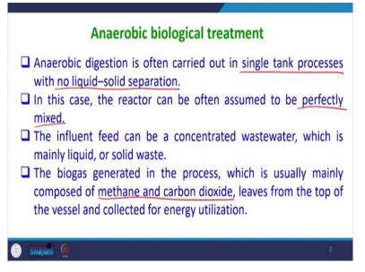
So, anaerobic biological treatment systems, they are often used and they are carried out the most of the treatment systems the treatment is carried out in a single tank process with no liquid-solid separation. So, this is the fundamental difference that there will be generally be carried out in a single tank process, in this case the reactor can often be assumed to be perfectly mixed.
