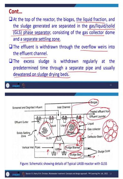
At the top of the reactor the biogas and the liquid fraction and the sludge generated are separated in a gas liquid solid phase separator, consisting of gas collector dome and a separate settling zone. So, we have a system of gas liquid solid separation unit which actually is a gas collector along with some area adjacent to the gas collector which works as a separate settling zone.
