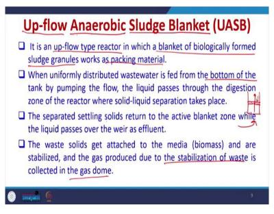
Now, within anaerobic treatment systems up-flow anaerobic sludge blanket reactor is one of the most common reactor and this can be used for the anaerobic treatment of wastewater. So, what is UASB reactor? It is an from the as suggested up-flow that means it is an up-flow type of reactor in which a blanket of biologically formed sludge granules worked as packing material, so this will understand.
