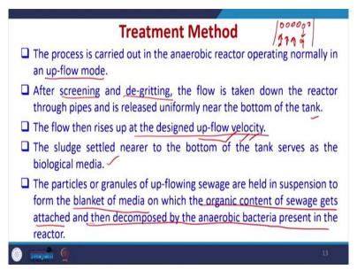
Now, how the treatment method works let us discuss this, the process is carried out in the anaerobic reactor operating normally in an up-flow mode. So, generally it will be up-flow
