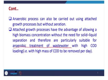
Anaerobic processes can also be carried out using attached growth processes but without aeration, so it is possible to use the attached growth processes without aeration for anaerobic treatment also. Attached growth processes have the advantage of allowing a high biomass concentration without the need of solid liquid separation and therefore are particularly suitable for anaerobic treatment.
