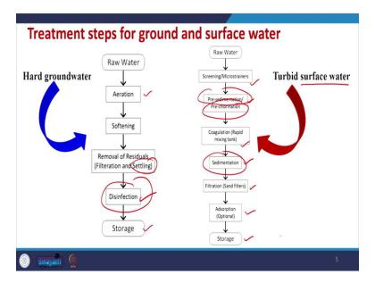
Now, there are various steps are unit operations which are performed for treatment of ground and surface water and this is done to get water for drinking or for other uses. Now, the wastewater treatment have certain steps, but the order in which these steps will be performed are different and they depend upon the characteristic of water which has to be treated.
