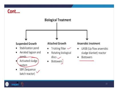
So, in the suspended growth, which are like aerobic methods, we can have a stabilization pond, aerated lagoon and ponds then activated sludge system which is the most common system then SBR the which is called sequential batch reactor and this SBRs are becoming now very common. Then attached growth systems like trickling filter, rotating biological, disc or bio towers may also be used.
