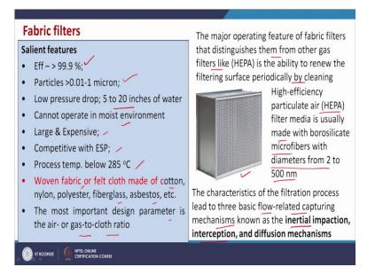
So, the salient features of these fabric filters are it is highly efficient 99.9 % or more than that efficiency is possible. It can be suitable for smaller particles also that particle size greater than 0.01 to 1 micron. Where the in case of settling we had seen that gravity settler it is more than 50 micron, but here it is 0.01 to 1 micron particle size can be separated and low pressure drop 5 to 20 inches of water.
