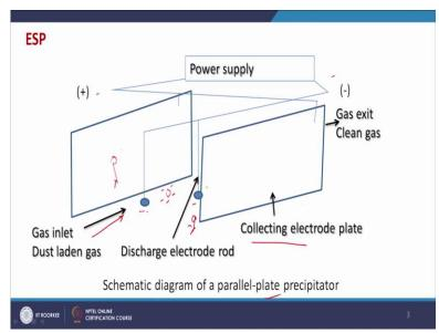
Now, we will see what electrostatic precipitators are. As you know, the particles are normally having negative charge. So, if we can create some electrical field through which the particle
