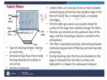
Now, we will discuss the fabric filters. So, you see this figure shows us the operation of fabric filters. So, here this is our dirty gas it is coming in and there are a number of stand we can see, these are the cages and these cage is covered by the fabrics or the bags. So, then this particulate matter leaden gas is coming here that is a dirty gas and it will be passing through the fabrics basically, there is one blower at the top. So, some suction is there.
