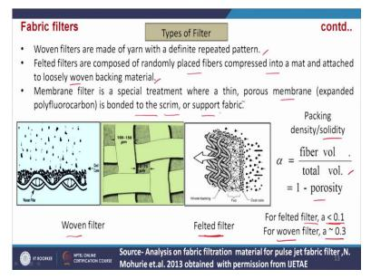
Now, we will see different types of filters and fabrics which are used in this type of filter. So, here you see the fibres are either woven or it is felted fibre. So, this it is very clear that in case of woven filtere, the volume of this fibre is much more than in case of filtered filter. So, the packing density is one parameter through which we can quantify the quality of these type of filters, so that packing density or solidity that is defined as
