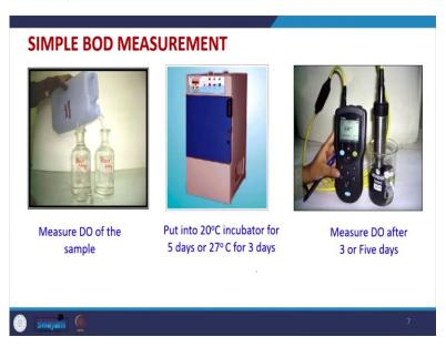
Now, these are the simple DO bottles and we can use this instrument for finding out the DO very easily.
