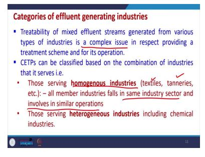
Categories of effluent generating industries already we have discussed. So, treatability of mixed effluent streams generated from various types of industries is a complex issue, it is not very, very easy with respect to providing a treatment scheme and for its operation. CETPs can be classified based upon combination of industry. So, homogeneous industries already we have discussed.
