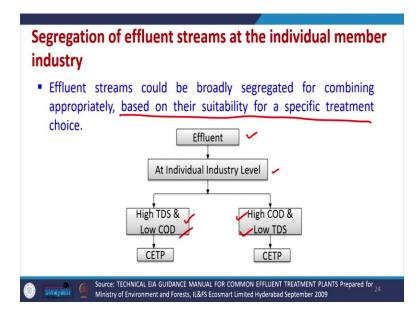
Now, before sending the effluent to the CETP, segregation of effluent streams at the individual member industry is also very important. So, effluent streams could be broadly segregated by combining appropriate based upon their suitability for a specific treatment. So, effluent at individual industry levels they may be classified into different high TDS, low COD or high COD low TDS. So, the treatment strategies could be different in the CETP for such wastewater. So, segregation is very important.
