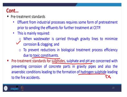
Now, the pretreatment industries effluents from industrial processes require some form of pretreatment prior to sending the effluent for further treatment at CETP. This may it is mainly required when wastewater is carried through gravity lines to minimize the corrosion and clogging to prevent the reduction in biological treatment process efficiency due to many any toxic constituents or otherwise.
