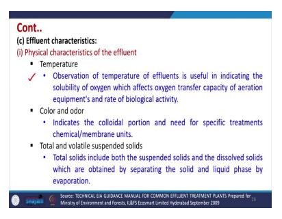
Now, in addition to flow rate, the quantity of water that will be generated the effluent characteristics is very very important. The physical characteristics of effluent in designing the CETP, which are very important include temperature. So, temperature of effluent is useful in indicating the solubility of oxygen which affects the oxygen transfer capacity in the aeration equipments. So, that is there.
