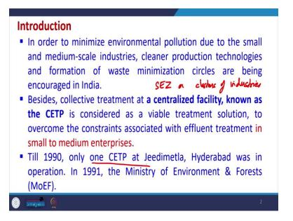
That means, wherever we have a special economic zone or wherever we have clusters of industries, so, at those places, the CETP is being made and the CETP which is a centralized facility, for that industrial cluster is being considered as a viable treatment solution. And actually, the use of CP helps in overcoming the constraints which may be associated with respect to effluent treatment in small and medium enterprises. So, it is there.
