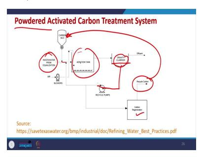
Then, we can have a powdered activated carbon treatment system within the refinery premises. So, wastewater after the equalization base in here and carbon from, so we have this is powdered activated carbon we may have a granular activated carbon bed we may have powdered activated carbon bed so, we have powdered activated carbon bed is used and in this particular unit, so we have this is getting mixed here.
