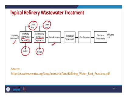
So, here we can see that refinery wastewater is coming. So, we may have primary oil water separation unit, which will remove the oil from the water then we may have secondary oil water separation unit against large and oil to oil will be separated out so, oil will be going to the top after that we have equalization basin followed by biological treatment clarification tertiary treatment and AOPs etc. So, this is there.
