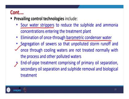
Now, the control strategies, what are the different prevailing control strategies? So, the sour water stripper is used to reduce the sulfide and ammonia concentrations entering the treatment plant. So, this is there. So, if it is done so, it is elimination of once-through barometric condenser water. So, this is done this eliminates this now segregation of severs, so that the unpolluted storm runoff and once through cooling waters are not treated normally with the process and other polluted.
