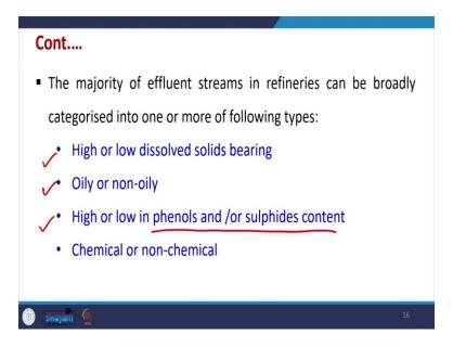
So, we need to treat such wastewater. So, the majority of effluent streams in refineries can be categorized into 4 of these types like high or low dissolved solids containing effluent then Oily or non-oily effluents, high or low in phenols or sulphide content, then chemical and non chemical type of compounds may also be present in the water.
