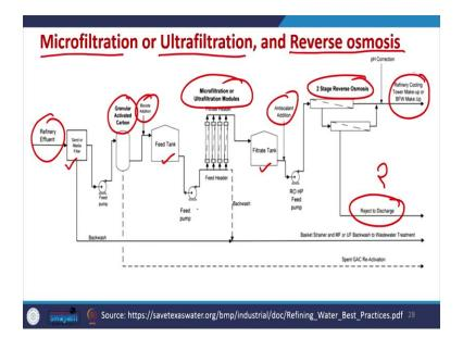
Now, effluent can also be treated in the micro filtration or ultra filtration and reverse osmosis unit in the petroleum refinery. So, the refinery effluent is first pass through sand or media filter. So, this is there and after that it is passed through the granular activated carbon. So, remember this is different than the powder activated carbon.
