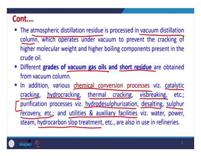
Now, the atmospheric distillation residue which is left it is further processed in the vacuum distillation column and it operates under vacuum certainly to prevent the cracking of higher molecular weight and higher boiling components present in the crude oil residue after the atmospheric distillation.
