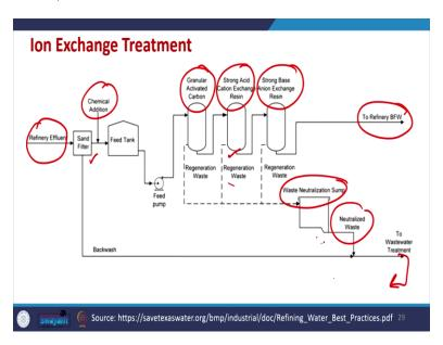
Then, we may have an Ion Exchange Treatment unit also. So, here the refinery effluent is coming, it goes into the sand filter as earlier after that some chemical addition is been done and it
