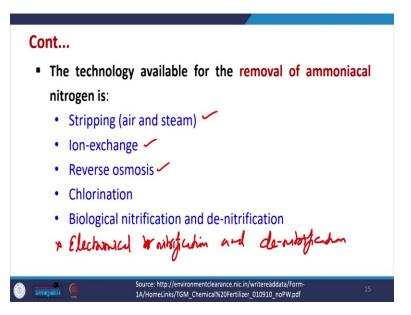
So, for doing this that technology available for removal of ammoniacal nitrogen includes a stripping, air and steam. Similarly, ion exchange units can be used for doing this. Reverse osmosis units have been used for treatment of such wastewaters, chlorination and biological nitrification and denitrification.
