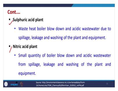
Similarly, in the sulphuric acid plant waste heat boiler blowdown and acidic wastewater due to spillage, leakage and washing from the plants and equipments may be there. For the nitric acid
