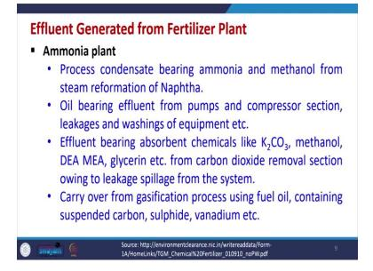
Now in the fertilizer plant without going much deeper into how the fertilizers are produced. There are different types of effluent that can be generated. So, the ammonia plant can generate effluent. (Refer Slide Time: 10:01)
