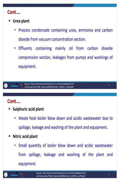
Similarly, there are other plants which can generate effluent including Urea plants sulphuric acid plant, nitric acid plant, single super phosphate plant, so, all these plants can generate different type of effluent. (Refer Slide Time: 10:09)
