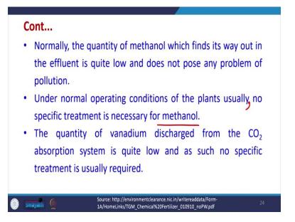
So, normally the quantity of methanol which is present in the effluent is low and does not cause that much problem. So, under normal operating plant a no specific treatment is done with respect to methanol but arsenic certainly we have to remove. The quantity of vanadium which is discharged from this system is also low and no specific treatment is required.
