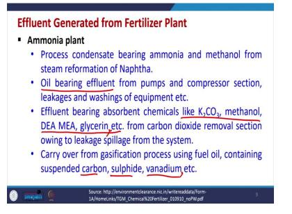
So, let us try to understand a little bit of the basics of this. So, ammonia plant, so, the process condensates bearing ammonia and methanol from the steam the formation of naphtha so, they may be present in the effluent which is generated from the ammonia plant then oil bearing effluent from pumps, compressors section, a leakage and washings of the equipment's etcetera will be present in this oil-bearing effluent.
