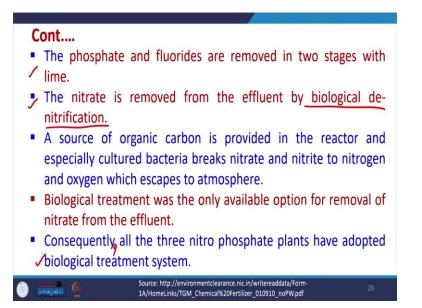
The phosphates and fluorides are removed in two stages with lime as we have discussed earlier. The nitrate is removed from the effluent by biological denitrification process. So, this is done. A source of organic carbon is provided in the reactor and specially cultured bacteria breaks nitrate and nitrite to nitrogen and oxygen which escapes to the atmosphere in this biological denitrification.
