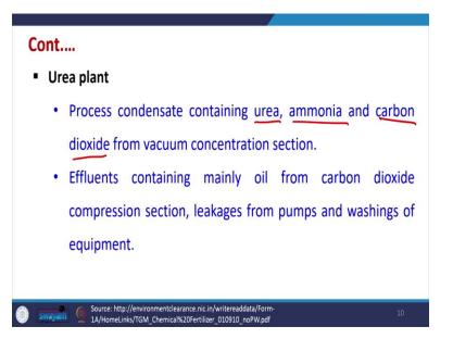
Similarly, Urea plant so, in the Urea plant process condensates containing urea, ammonia, carbon dioxide from vacuum concentration unit may be getting generated and that will be containing these compounds. Similarly, effluents containing many oil from carbon dioxide compression section, leakages from pumps and washing of equipment's may be present in the Urea plants so, these effluents may get generated in the Urea plant.
