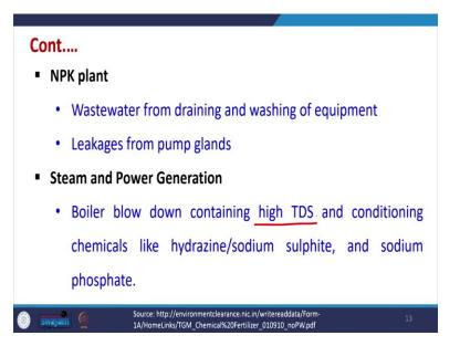
Now NPK plant the wastewater from draining and washing up equipment and also from leakages from pump glands etcetera. will be there. In the steam and power generation unit also, the boiler blowdown containing high TDS and conditioning chemicals such as hydrazine, sodium sulphite and sodium phosphate may get generated.
