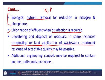
Then also because lot of nutrients are present in the sugar industry water, so, nitrogen phosphorus, etc., may be present. So, we have to see the biological nutrient removal for reduction in nitrogen and phosphorus is done, and in India the sugar industry wastewater is allowed to be used in the field also for irrigation after treatment up to a certain value. So, there also we can be and this is because the sugar industry wastewater contains large amount of nutrients.
