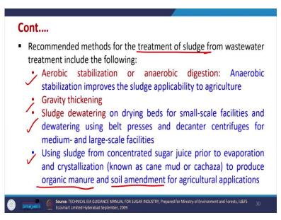
Recommended method for treatment of sludge from wastewater treatment include aerobic stabilization, gravity thickening, sludge dewatering and using sludge from concentrated sugar juice prior to evaporation and crystallization to produce organic manure and soil amendment for agriculture applications. So, this is how the, we have to take care of the sludge which is generated in the wastewater treatment plants, so this is there.
