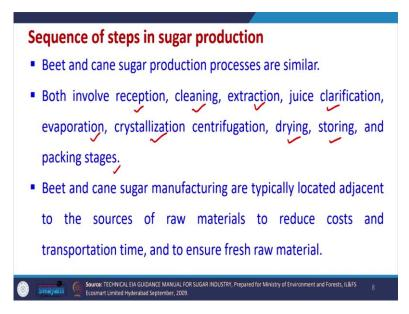
So, these are the different steps which are followed in this sugarcane production. Now, the sequence of steps in the sugar production are given here. So, the beet and cane sugar production processes are in very similar, both involved reception, cleaning, extraction, juice clarification, evaporation, crystallization, centrifugation, drying, storing and packaging.
