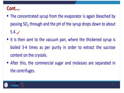
So, these are the steps. The concentrated syrup which is obtained from the evaporator is again bleached by passing sulphur dioxide through it and the pH of the syrup drops to about 5.4. Then it is sent to a vacuum pan, where the thickened syrup is boiled 3 to 4 times as per the purity in order to extract the sucrose content of the crystal in the form of crystals, after this the commercial sugar and molasses are separated in the centrifuges and then used further on.
