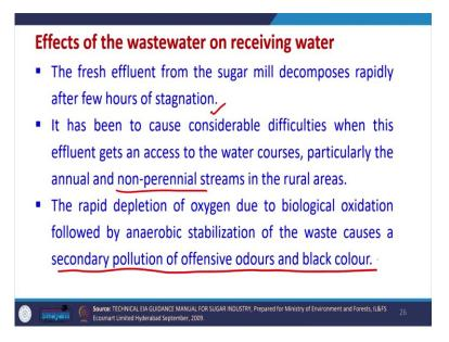
Now, for sugar industry, it is allowed the water after treatment is allowed to be used in the adjoining irrigation, adjoining field for irrigation. The fresh effluent from the sugar mill decomposes rapidly after few hours of stagnation, and it has been to cause considerable difficulties when this effluent gets an access to the water courses, particularly annual or non-
