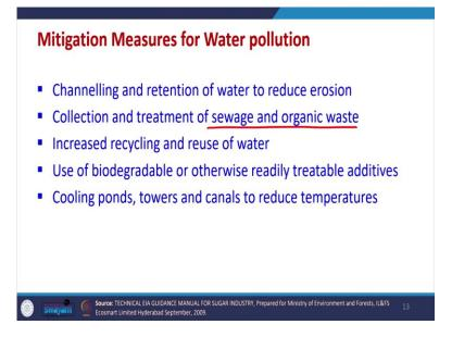
So, these are the characteristics of water which are discharged from different section. So, what are the mitigations measures that are generally taken in a sugar industry. So, channeling and retention of water to reduce the erosion, so, this is their. Collection and treatment of sewage and organic waste. So, this is also done because a number of people are working in the industry.
