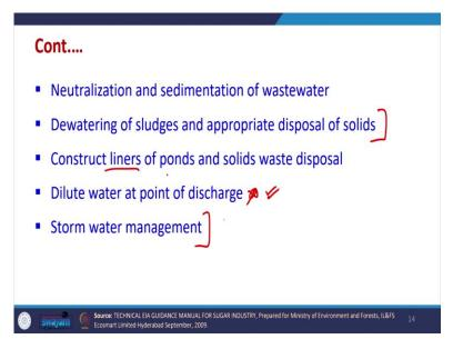
Construct liners of ponds and solid waste disposal units all in these units we have to construct liners also, dilute water at point of discharge if it is there, this is dilute with the already some other water which may be there which has to be treated. So, this then storm water management, this is not what is preferred. So, this is always the water has to be recycled, if it is beyond a certain value and it has to be treated further.
