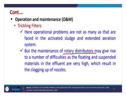
Similarly, for trickling filter also, all the operational problems are similar, but are not as many as that are there in the activated sludge process or that aeration unit. The maintenance of rotary distributors which are there on the top of trickling filter that is one of the problematic areas. So, we have to take care of that.
