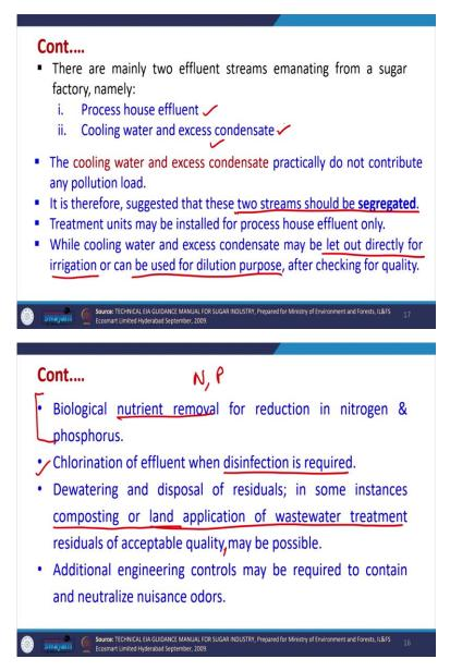
There are mainly two effluent streams emanating from the sugar industry. So, we have process house effluent and cooling water and excess condensate. So, the process water treatment already we have discussed the cooling water and excess condensate which is there that they do not have any pollution load.
