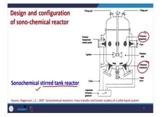
So, Sonochemical stirred tank reactor this is this technology is not much practice react in large scale reactors, but these are the different types of reactors which have been reported. So, we can see here this is a stirred tank reactor, but along with some Ultrasonic transducers which are fitted for generating the bubbles and then the using that cavitation effect. So it is very common a stirred tank reactor but it is fitted with Ultrasonic transducer.
