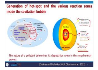
Now, let us further understand the generation of hotspot and the inside of the cavitation bubble and their various reaction zones etc. So, this is shown. So, we have three already discussed we have three zones, we have cavity interior. So, it is a considered as a volatile hydrophobic substance a temperature and pressures are already given.
