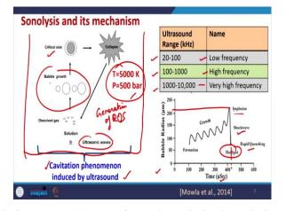
So, we use basically <u>ultra soundultrasound</u> for creating cavitation So, cavitation means creating bubbles. So, this idea is used for generation of reactive oxidation is species and which are further used for treatment of the water. Sonolysis can be used individually also it can be used along with some other advanced oxidation processes, including electrochemical treatment and <u>photo lysisphotolysis</u> where via combining this Sonolysis we actually enhance the treatment
