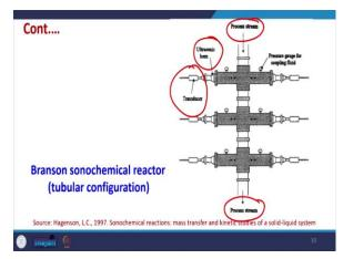
Similarly, this Branson Sonochemical reactor has been reported. Again we can see that transducers and Ultrasonic horn here the process is stream to the water to be treated is coming in after treatment it is going like this. So, this is again a tubular configuration of <u>Sonochemical</u> reactor, which has been reported.
