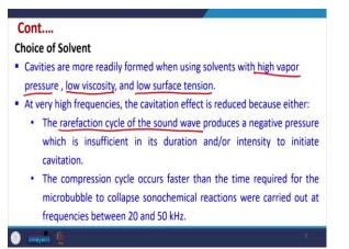
So, this is there now, choice of solvents. So, depending upon what type of solvent or what type of other types of materials which are present in the water that will also affect the Sonolysis cavities are more readily found when using solvents with high vapor pressure, low viscosity and low surface tension.
