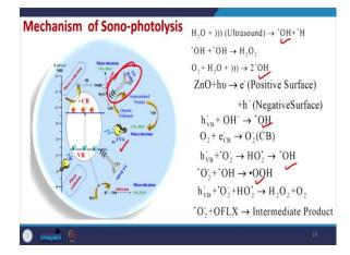
So, this is how the Sono photolysis works. Generally, it will combine along with the Hv. So, we have both light and sound transducers both are there. So, because of that, there is increased formation of radicals and because of quick formation of radicals, we have more treatment, which happens and because of which that treatment efficiency becomes very, very high.
