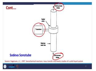
This is an another Sonotube where transducer is fitted. So, again a simple transducer is being fitted in the line itself. So, here we have inlet processes team and here the outlet processes stream is there where the water is coming out after the treatment. So, these are the various configuration of <u>Sonochemical</u> reactor.
