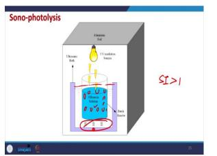
Now, Sono-photolysis is another technique. So, here we can see this treatment is being done in a batch reactor Ofloxacin solution and we have this it contains already photocatalysis and UV light is being provided. So, we have photocatalyst which are here and then the photo oxidation is happening, but if we use Ultrasound, so it will increase the efficiency and SI value is likely to be greater than 1. So, this is also possible in Sono photolysis.
