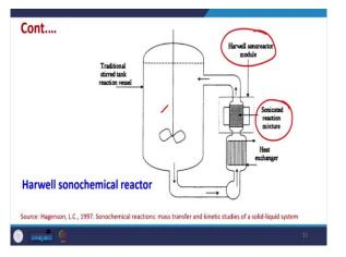
Similarly, a harvest, Sono chemical reactor has been reported where the recycling is being done and the water from the stirred tank vessel is coming and then it the reaction is being done separately out of the reactor and here the <u>Sonochemical</u> reaction mixture here this Harwell Sonoreactor module has been acted and water is further edit and treatment is being done in the usual CSTR method.
