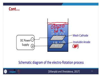
So, we have electrodes, we can see, the mesh electrodes, insoluble electrodes. So, that means these are DSAs. So, if DSA is dimensionally stable anodes. So, from here the O2 or H2 evolution is taking place and these bubbles when going up, they will interact bigger particles or other organic compounds and they will react with these bubbles and they will be taken and we have a foam layer which will be formed at the surface, so, this is there.
