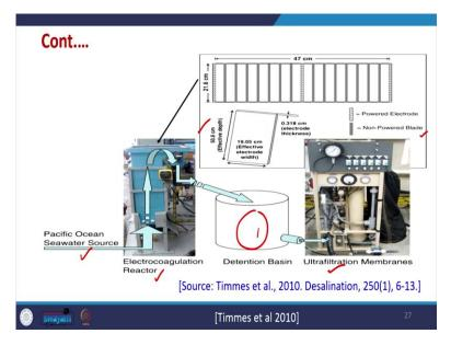
So, this is another which is reported, so, this is like Pacific Ocean sea water source, so electro-coagulation is being performed and after electro-coagulation there is some detention basin is which is there. So, the setup of electrocoagulation is given here, so, electrodes we can see a number of powered electrode and non-powered blades are there within this electrode configuration and after that this is being further treated by ultrafiltration membrane.
