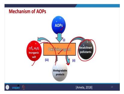
So, we have recalcitrant pollutants. So, various AOP techniques are there. So, they will get converted into biodegradable products in the presence of oxidizing agents, which are getting generated because of these AOPs. And then these biodegradable pollutants are converted into these CO2, H2O, inorganic salts etcetera. So, this is the mechanism of AOP and how it works.
