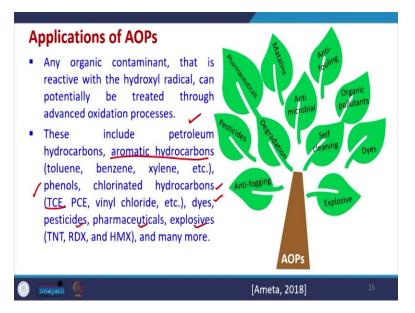
Now, AOPs can be used for treatment of many types of organic contaminants. So, this is here. And they are, since they are non selective they can be used at many places. So, the type of wastewater which can be treated using AOPs include like petroleum hydrocarbons, aromatic hydrocarbons (toluene, benzene, xylene, etcetera). Since, phenols, chlorinated hydrocarbons like PCE, TCE, vinyl chloride, etcetera.
