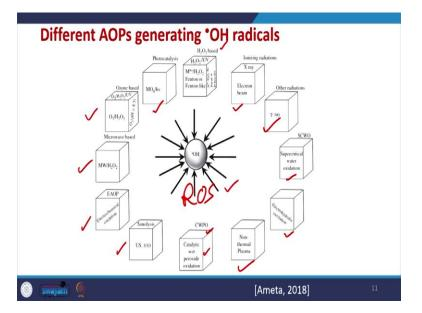
Now, these are different AOP generating OH radicals, AOPs, which generate OH radicals or any other reactive oxygen species by different means, the same we can use photo-catalysis, we can use lot of hydrogen peroxide based techniques which is called as per oxidation. So, we can use hydrogen peroxide along with some catalyst. So, they will always produce reactive oxygen species.
