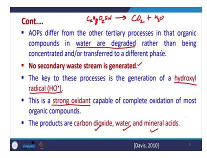
They are able to remove the suspended solids, organic matter, nutrients etcetera and that are undesirable in any of the water or wastewater. Now, with sustainability coming into the human life, as well as the growth with industrialization, there are many pollutants which are coming into the water and these pollutants include those like pharmaceutical pollutants, personal care products, many of them are endocrine disrupting chemicals.
