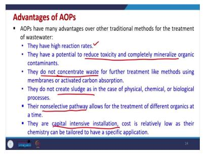
The advantages already we have discussed few of them, but there are other advantages also over traditional methods for the water treatment. So, these AOPs generally have high reaction rates. So, that means, the reactor configuration will be smaller. So, higher the reaction rate the faster will be the treatment. So, within a reactor volume, we can treat more amount of water or if the amount of water is fixed per unit hour how much it is generated, we can reduce the reactor volume.
