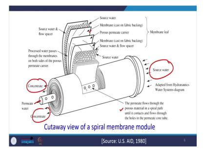
Now this is a cut away view of spiral membrane module you can see here. These are the different, so source water we can see here the permeate will be coming out from here. The
