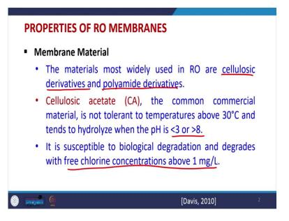
So, membrane materials, the materials most widely used in the RO like cellulosic derivatives are polyamide derivatives. So, these are very very common materials which are used as RO membrane material and cellulose acetate the most common commercial material which is used in the membranes for RO is not tolerant to temperatures above 30 degree centigrade and tends to hydrolyze for the pH range which is beyond three and eight.
