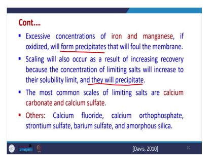
Excessive concentrations of iron and manganese, if they are present in the water and if they are oxidized. So, what will they do is that, they will form precipitate and that will follow the membrane. So, this is there. Scaling will also occur as a result of increasing recovery because the concentration of the limiting salts will increase to their solubility limit and after that they will start precipitating. So, this is another reason for fouling or scaling.
