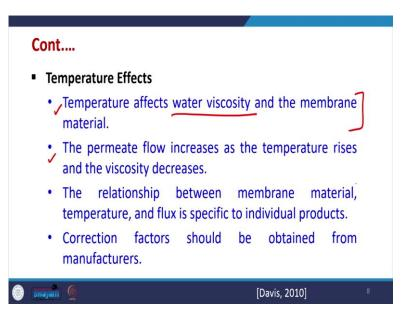
Now there are different effects which are there. So, earlier we have seen that the temperature affects the membrane performance of ultrafiltration, nano-filtration and microfiltration. For reverse osmosis case also it is the same because the temperature affects the water viscosity and as well as the membrane material also. So, we have seen with respect to cellulose acetate that temperature there is the effect of temperature on the cellulose acetate material.
