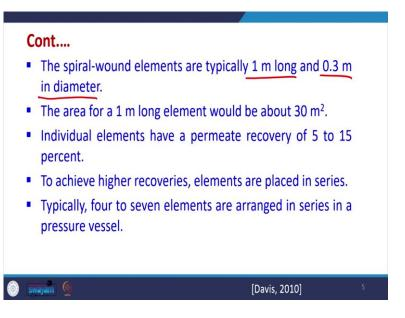
Now the spiral wound elements are typically one meter long and 0.3 meter in diameter. So, this is there. This is a typical configuration of spiral wound element. Now the area for one meter long element will be typically 30 meter square. Individual elements may have permeate recovery of 5 to 15 percent. To achieve higher recoveries these maybe placed in series also and typically 4 to 7 elements are arranged in a series in a pressure vessel. This is how the recovery rates are increased.
