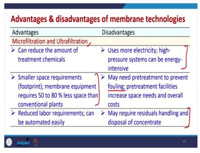
Now, we will try to understand the advantages and disadvantages are different membrane technologies. So, for microfiltration and ultrafiltration the advantages and disadvantages are
