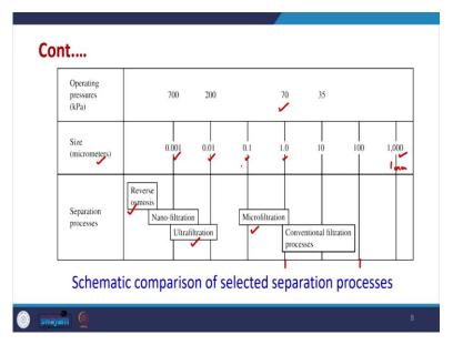
Now, these processes, they work for different operating pressure, different size of constituents they can remove, and so, they work in different pressure range and size range. Now, so, this is what is given here. So, we can see the size range in micrometres. So, as the size range increasing, so, you can see here, it is like one millimetre size here.
