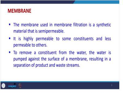
Now, the membrane used in the membrane filtration is a synthetic material. So, that is semipermeable. So, semipermeable means that it will generally allow the water to pass through it, but it will not allow other materials to pass through it. So, it will be like a filtering system for some of the material, but it allow some other material to pass through it.
