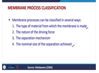
Now, membrane processes can be classified into via several ways. So, that will depend upon the type of material from which the membrane is made. So, this is one thing. So, that will depend upon that how much pressure has to be sustained, what type of constituents have to be removed. So, we can have some functionalities which are there on the membrane itself, that will help in the degrading some of the pollutants and filtering some of the pollutants.
