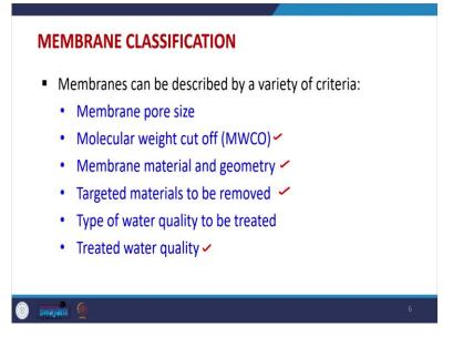
And membranes themselves can be described by a number of criteria. So, one thing is the classification of membrane processes, another is how membrane themselves can be classified, or described? So, for describing any membrane, we use a number of parameters, and those parameters include the membrane pore size, this is the most important criteria, that what is the size range under with different membrane processes are being operated.
