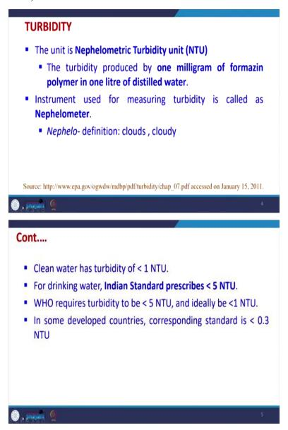
Now, turbidity is measured using an instrument, which is called Nephelometric turbidity unit and this actually that turbidity produced by one milligram of for formazin polymer in one liter of distilled water. It is said to be this is the unit and it is equal to one NTU. So, one NTU is like one milligram of formazin polymer dissolved in one liter of distilled water.
