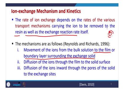
Now, what are the different ion-exchange mechanism and kinetics? So, the rate of ion exchange depends upon the rates of various transport mechanisms, which get carried out in the bed. And depending upon the ion to be removed, and how the ion moves towards the resin and how quickly or how faster the ion-exchange reaction takes place. So, a number of parameters are there. Now, there are different steps within the mechanism.
