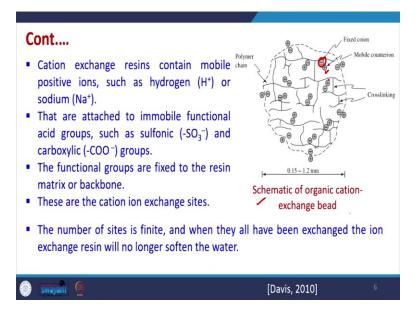
Now, cation exchange resins contain mobile positive ions such as hydrogen or sodium. So, they are attached to the immobile functional acidic groups such as sulfonic or carboxylic group. So, this plus charge will be always be attached to this minus charge. Now, the functional groups are fixed to the resin matrix or the backbone. So, this is there. And these are the cation ion-exchange sites.
