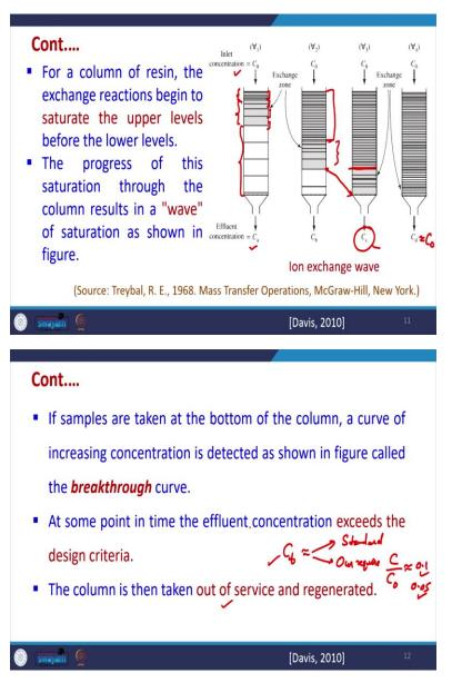
Now, for a column of resin, the exchange reactions begins to saturate the upper levels first before the, so suppose the flow rate is from the top. So, initially this zone will be utilized then this zone then this zone. So, we can see here the moment this is like mass transfer zone in the adsorption. So, in the effluent concentration is coming out Ca here and inlet concentration is C0.
