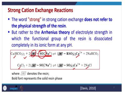
Now, going further there are strong cation exchange reactions which are possible. So, strong here does not mean that the physical strength of the resin, here it means that with respect to functional group. So, rather to the, like what type of functional groups are there and whether the cation exchange how much cation exchange is possible, we can, can we replace all the cations or not. So, all these things are there.
