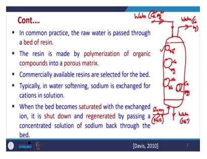
So, in common practice, what is done is that, suppose, we have this bed is there. So, we will be having a bed, packed-bed similar to the adsorption. So, suppose this is the bed and we have some water which is coming and that water is there and that water is containing suppose calcium, magnesium, etc. So, this is there. So, calcium Ca2 plus, Mg2 plus will be there.
