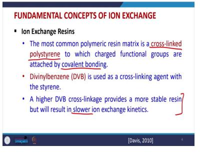
Now, there are some fundamental concepts for ion-exchange. So, one of the most important thing is ion-exchange resin. So, which type of ion-exchange resin has to be used or which type of, that depends upon the ions that have to be exchanged. So, the most common polymeric resin metrix is like a cross-linked polystyrene to which different charged functional groups are attached by covalent bonding.
