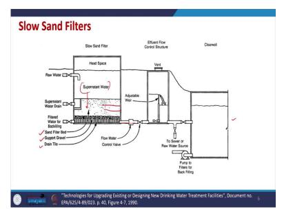
This is how slow sand filtration is there, raw water is coming. So it will be here and then it will be percolating we have different types of beds you can see, so, we have sand filter bed, support gravel, then there is a, grey, drain tile is there, we can have multiple beds also here, possible of different filter media, so this is there.
