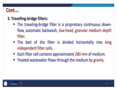
Similarly, there is another type of depth filter which is called as traveling-bridge filter. And again it is a proprietary continuous down-flow automatic backwashing, low-head, granular medium depth filter, we can go and cross-check these filters in detail if you are interested. The bed of the filter is divided horizontally into long independent filter cells.
