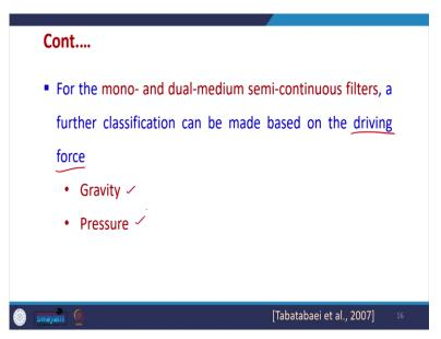
Also for the mono and dual medium continuous, semi-continuous filters, a further classification may be with respect to the driving force. So, it may be possible the flow is via gravity and or some pressure has been applied. So, both possibilities are there. So, if via
