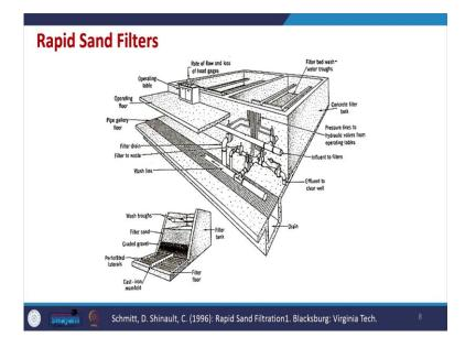
And this is the diagram of Rapid sand filter. And so, we have different components within this Rapid sand filter including like wash lines, filter Drain, filter to waste, operation is very similar to that only the rate of operation is faster.
