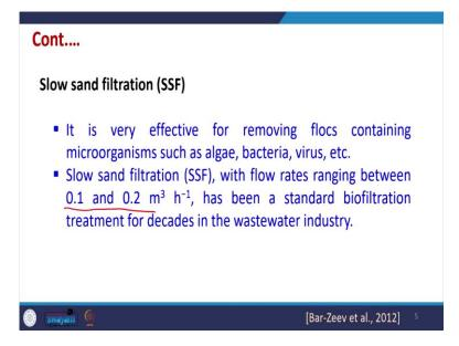
Now, continuing one of the first unit which is very common, it is called slow sand filtration. So, it is very effective in removing flocs containing microorganisms such as algae, bacteria, virus, etc. And slow sand filtration generally operates in the range of 0.1 to 0.2 meter cube per hour. This is the usual which is common, and if the flow rates are higher or otherwise, we can have a multiple units in parallel, so this is there.
