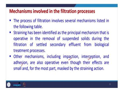
Now, these mechanisms may include single mechanism or a combination of mechanism, so, they may include, simple filtration mechanism in addition to that, they may have, impaction, interception, adhesion. So, all these are possibilities which are there during the filtration all these mechanisms may also be occurring. So, let us try to understand this what are the different mechanisms.
