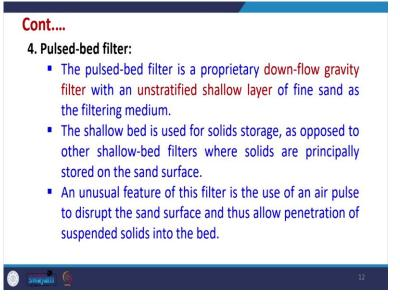
Then we have a pulsed-bed filter also. So it is a proprietary type of filter and it has a unstratified shallow layer of fine sand as the filter medium. The shallow bed is used for solid storage, as opposed to other shallow bed filters where solids are principally stored on the sand surface, but here there is a shallow bed which is used for the solid storage.
