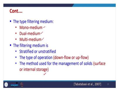
Similarly, based upon the type of filter medium, we can have mono-medium, dual-medium or multi-medium filtration, which are possible. The filtering media can be stratified, unstratified. The type of operation the flow may be down-flow, up-flow, the method used for management of solid maybe surface it may be only captured on the surface, it may be some possibility of internal storage may be given. So, these are the different ways in which the filter mediums can be classified.
