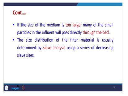
So, there is a situation that we have to properly select the size of the medium neither we can go for too small, where the head loss will become very high or too big, where the particles are not filtered at all, this is the possibility. The size distribution of filter medium is usually determined by sieve analysis or a number of other methods can also be used, this is the possibility.
