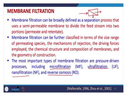
Now, there is a second type of filtration which is, which we will be discussing only a little bit, it is called as Membrane filtration. So, it can be broadly defined as a separation process in which a semi-permeable membrane is used to divide the feed stream into two portions, and which is called as permeate and retentate. So, a membrane filter can, we have two streams which are divided because of these membranes which will be there, so, it is possible to have such type of unit.
