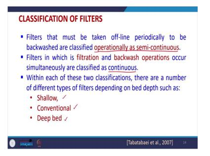
Now, classification, these are the simple classifications, there can be other classifications also, like if the filters that must be taken off periodically to be backwashed. So, they can be classified as semi-continuous, because we have to go for backwashing, so, they are not continuous.
