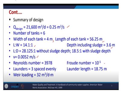
So, overall design was that, that the flow rate was this 21,600-meter cube per day or 0.25-meter cube per second, the number of tanks were 6 and the width of each tank has been taken as 4 meter, length has been taken as 56.25 meter, the L by length width ratio was this and depth including the sludge zone etcetera was 3.6 meter and the overall without considering the sludge depth.
