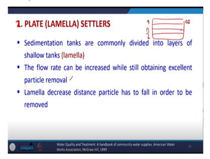
Now, second of the, this high rates settler is the plate or lamella settler the sedimentation tanks are commonly divided into layers of shallow tanks so, what is done is that? Overall the sedimentation basin may be like this, D is the depth now, what is done is that, this is divided into a number of layers, so, depth has decreased. So, it is now D1 only if you consider like this, so, the depth will decrease.
