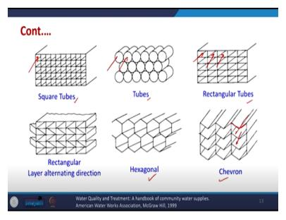
So, these are the different cross-sections which are possible square tubes, these are simple circular tubes, then we have rectangular tubes, rectangular with layers alternating the direction so, we can see here some layers are also there in between we have hexagonal or chevron type where there is some inclination is there so the sludge may easily settle and come out here in chevron tubes, these are all possible.
