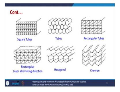
So, you can see the pictures here. So, through this the water to be processed will pass in any of these tube settlers and they may be of different dimensions. So the water has to pass through them.
