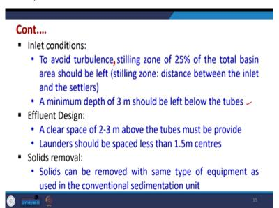
Now, in the inlet condition to avoid the turbulence stilling zone of around 25 percent of the total basin area should be left. So, this is there. So, to avoid this turbulence we had to take care of this and minimum depth of 3 meter should be left below the tubes. So, this is another one of the from experience this criteria has come. Now effluent design a clear space of 2 to 3 meters above the tube must be provided. Launder should be placed less than 1.5 meters on the center. So, this is there.
