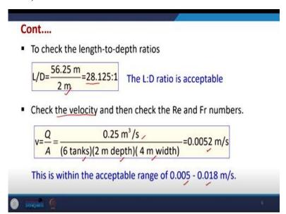
Now, the, now cross-checking with respect to length to depth ratio, it is 56.25 and 2 meter because actual water depth is only 2 meter, 1 meter is for the sludge depth. So, side water depth was 3 meter, now, the actual depth is where the water or settling etcetera is occurring is 2 meter. So, under that condition the ratio is 28.125 is to 1 and this may be considered as acceptable.
