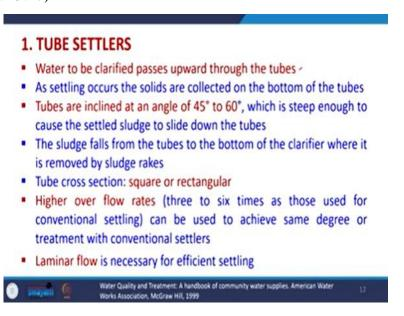
Now, understanding each of them one by one so, first is the tube settler. So, water to be clarified passes upwards through the tube.
