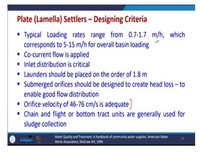
Now, some design criteria is that the typical loading rate range from 0.7 to 1.7 meter per hour which corresponds to 5 to 15 meter per hour for overall basin loading. So, we have to take care this. Co-current flow is applied, then inlet distribution is very critical and that has to be taken care.
