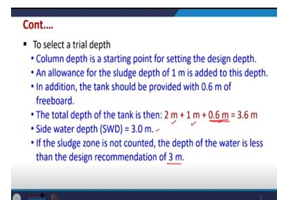
So, this is taken now, we have to take the trial depth, so, the column depth is a starting point for settling of the, for designing the settling basin. So, an allowance for sludge depth of 1 meter is recommended. Now, in addition the tank should be provided with 0.6 meter of the freeboard above, so, that also has to be taken care. So, since the depth was 2 meter for the column and we may start from there itself.
