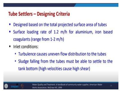
Some design criteria for tube settlers are there is that the design is based upon the total projected surface area of the tube. So, this is important already we do this. The surface loading rate of
