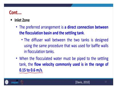
Now, in Inlet zone the preferred arrangement is that a direct connection is there between the flocculant basin and the settling tank. So, this is what is the preferred arrangement. A diffuser wall between the two tanks is designed using the same procedure that is used for baffles walls in a flocculant tank. So, we can use the same technique. Now, when the flocculated water is piped to the settling tank, the common flow velocity which is used is in this range from 0.15 to 0.6 meters per second.
