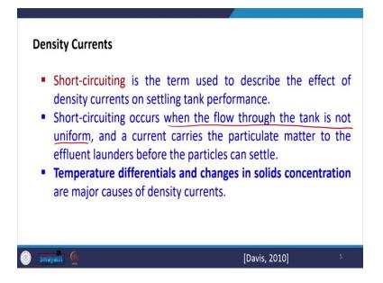
Then the second parameter is the density current. Density current is like it happens because of the effect of various effects, it may be because of the variation in the density, it may be also because of the variation in temperature. So, temperature variation changes in solid concentration all may cause the variation in density and that density may lead to density current and density current actually leads to the short circuiting.
