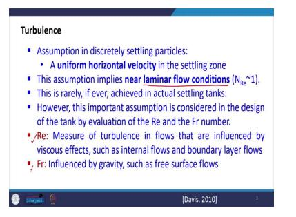
Now, starting with the turbulence, so, suppose, we are assuming a discrete settling particle and in this condition what we assume is that in the basin it has a uniform horizontal velocity in the settling zone. Now, this if we consider this assumption, this will this will be like assuming that laminar flow conditions are there inside that settling zone.
