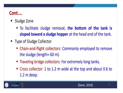
Now there are different types of sludge collectors. So, once it moves to the sludge collector, we may have different types of sludge collector. So, chain and flight collectors are there, so they are commonly applied to remove the sludge, the length is approximately 60 meter or maybe others
