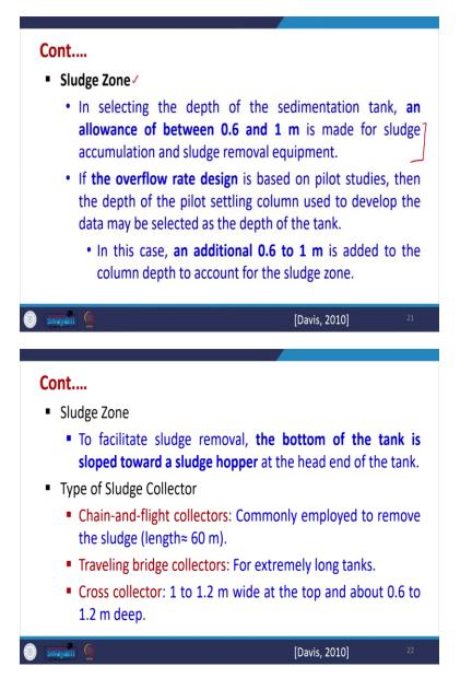
Now, sometimes we may use an additional 0.6 to 1 meter to the column depth to account for the sludge zone. So, this is also possible so sludge zone is very important. And to facilitate easy sludge removal, the bottom of the tank is sloped towards the sludge hopper and head end of the tank.
