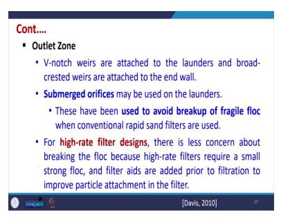
Now, in the outlet zone, we have V notch weirs, which are attached to the launders and they and broad crested weirs maybe attached at the end wall. So, this is there. Sometimes we use submerged orifice may be used on the launders and they have been used to avoid the breakup of fragile flocs, when conventional rapid sand filters have to be used later on. So this is good if the suppose we have a fragile floc and in the floc is bigger.
