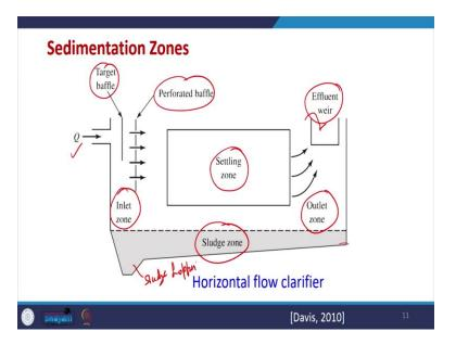
So, we can like here in the figure you may have seen this is slanted and this is the sludge hopper which is there. So, we have to see that this is slanted and we can easily remove the sludge whenever desirable. So, this is there. So, this is what is written here in the.
