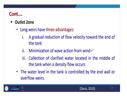
Now there are other there are certain advantages of using long Weir's. So, these advantages are like a gradual reduction of flow velocity towards the end of the tank. So, this is possible. So, that is if we use long weir it is possible then we have we can minimize the wave action from wind. So, we are taken care of the wind also by using the long weirs.
