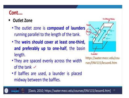
Now, after settling we have outlet zone, the outlet zone is composed of like launders running parallel to the length of the tank. So, this is there and the weirs after the settling zone, they should cover at least one third or one half of the basin length. So, that has to be taken. So, we can see that we are here and we have the notch here.
