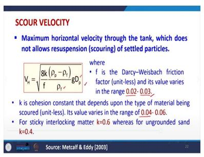
Maximum horizontal velocity through the tank, which does not allows resuspension (scouring) of settled particles.
