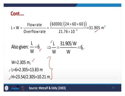
Now, going further similarly the surface area of the tank is equal to flow rate divided by overflow rate and that comes out to be 31.905-meter square so we calculate it. Now, since L by W was taken as 6, so L by W is equal to what we do is that we put the from here the term for L so from here L will be equal to 31.905 divided by W so this is there.
