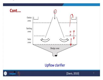
Similarly, for Upflow clarifier also the inlet is from the top and then it is getting distributed from here. And the particles get settled down particles those particles which will be there actually they will be settling down and reaching the sludge zone. And ultimately the treated water containing smaller amount of particles will be going into the outlet zone and going out so this is there. So, we have horizontal flow clarifier we have up flow clarifier so we will go further and discuss this.
