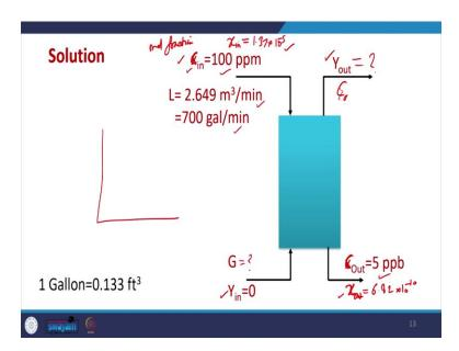
Now if we perform the, this is 100 ppm Cin. So, we have to find out the Xin. So, Xin is being found out here. So, 100 ppm is being converted into mole fraction. So, this is first step, similarly, 5 ppb, which was given here it is being converted into mole fraction. So, both the mole fraction at Xin is known and X actually this is C out. So, we have X out is known to us and this has been calculated in this slide.
