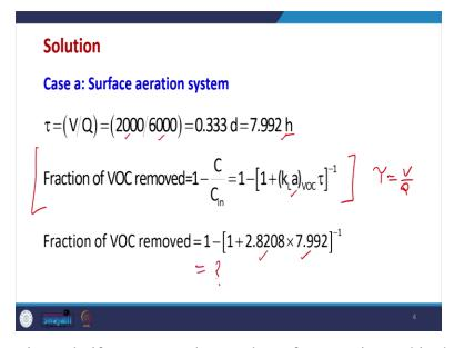
So, for surface aeration only if suppose we have only surface aeration and in the second case we have only diffused aeration. So, first step is to find out the KLa value if you remember, the equation for surface aeration was this and within this that tau value is given by V by Q. So, this this was the equation that we derived in the previous class.
