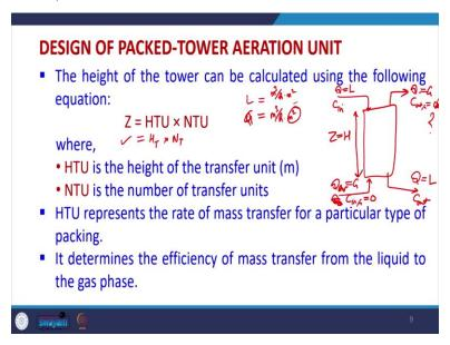
So, this is a simple packed tower aeration we may write like this. So, water is coming here, it will be having some concentration of pollutant and this water will go out from here and its concentration will be reduced a certain value will be having a air. So, we can write for air some flow rate, it will be certainly having no VOC concentration initially and then it will be going out at certain air flow rate.
