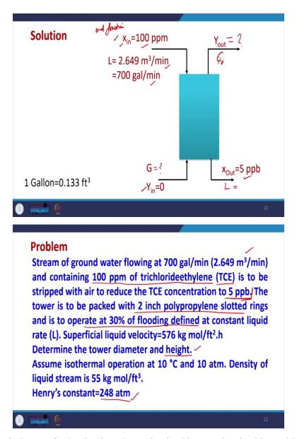
Now, let us put a balance of what is given here. So, in this equation in this problem it is given to 2.649 metre cube per minute is the flow rate okay in gallons also because gallons is the common terminology in many countries. So, we can calculate in gallons also, but we are writing like this only. So, this is the flow rate and this is the 100 ppm, but we want it to be reduced at 5 ppb. So, here L will be the same.
