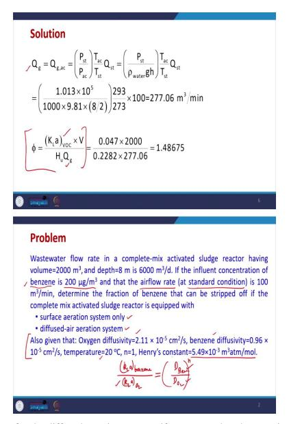
In the second case for the diffused aeration system, if you remember the equation was given like this that the final equation was like this, we derived and for solving this we require Hu, we require this psi and this psi itself is given by this particular equation and in this KLa is also required.
