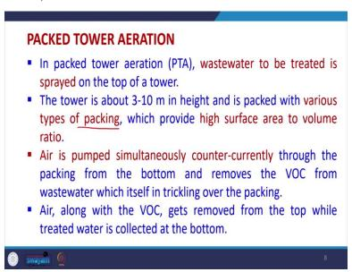
Now, going further there is another type of aeration which is very common it is called packed tower aeration. So, in the packed tower aeration wastewater which is to be treated is sprayed on the top of the tower and the tower height may be anything from 3 to 10 metre a little higher a little lower and is packed with various types of packing.
