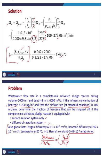
Now, this equation can be changed. So, Qg is actually equal to Qg ac and this is the equation. Now, we are what we are doing we are assuming this both the temperatures to be same. So, no, no, here at the standard condition it is given 200, 100 metre cube per minute. So, at a standard condition it is 273 degrees centigrade and here we have to calculate at 20 degrees centigrade it is 293 kelvin.
