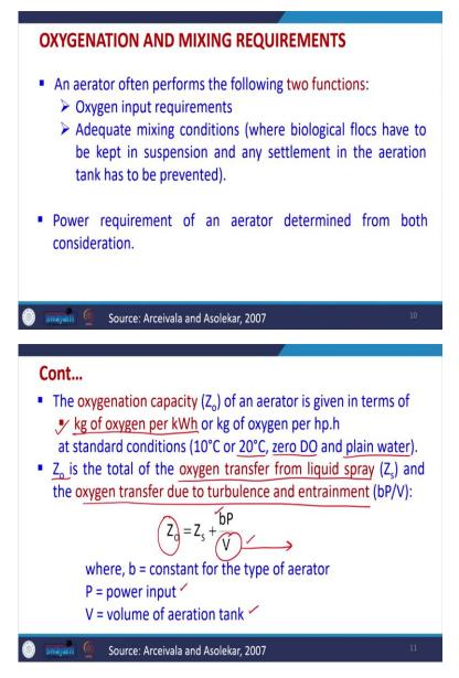
So, how much amount of oxygen we require? So, this is the most important consideration for aerator. So, this is there and we should calculate the power rating depending upon that. Second thing is that how much mixing has to be done. So, it will be more correct for aerators like process where some treatment by biological microorganisms is being done. So, how much mixing is essential because if mixing is not there, so, the pollutants are not coming in contact with the microorganisms.
