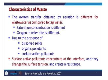
Then a characteristic of waste. So, type of waste in which the aeration is going to be carried out. So, this is very, very important and it actually affects the oxygen transfer rate a lot. There may be a number of components which may be present in the water and that may be hydrophobic, hydrophilic, there may be some type of surfactants which are present and so, all those things actually they add on additional resistances in the water. So, and that causes a lot of problem.
