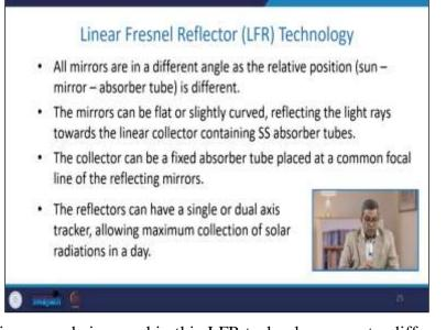
So, whatever mirrors are being used in this LFR technology are at a different angle as the relative position that is a sun mirror, or absorber tube is different. These mirrors can be flat or slightly curved, reflecting the light trays towards the linear collector containing stainless steel absorber tubes. The collector can be a fixed absorber placed at a common focal line of the reflecting mirror.
