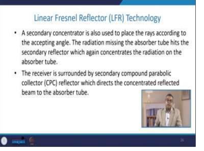
And usually, the receiver is surrounded by a secondary compound parabolic collector (CPC), which directs the concentrated reflected beam to the absorber tube.
