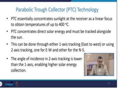
So, first is the parabolic trough collectors technology PTC. The PTC essentially concentrates sunlight at the receiver as a linear focus to obtain a temperature up to 400 degrees Celsius. It concentrates direct solar energy and must be tracked alongside the sun. So, the moment alongside the sun needs to be tracked. This can be done by either one axis tracking east to west or using two excess trackings, one for east to west and the other from north to south.
