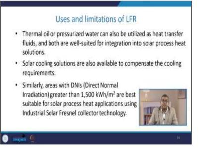
Thermal oil or pressurized water can also be utilized as a heat transfer fluid, and both are well suited for integration into solar process heat solution. So, solar cooling solutions are also available to compensate for the cooling requirement. Similarly, when we talk about the direct normal irradiation which is greater than 1500 kilowatt-hour per meter square at
