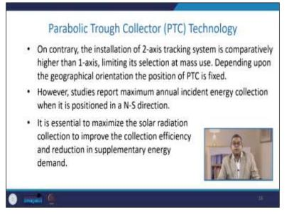
On the contrary, installing a 2-axis tracking system is comparatively higher than one axis, limiting its selection at mass use. Depending upon the geographical orientation, the PTC position can usually be fixed. However, studies report the maximum annual incidence to incident energy collection when it is positioned in the north to south direction.
