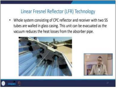
The LFR technology whole system consists of a CPC reflector and receiver with two stainless steel tubes walled in a glass casing. You can see this tube, and this is the glass casing. This unit can be evacuated as the vacuum reduces the heat loss from the absorber pipe. So, these are the absorber pipes, and if you put a vacuum, the heat loss can definitely be minimized.
