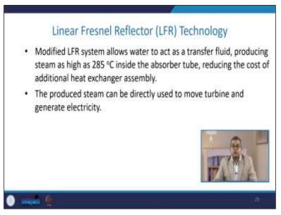
The produced steam can be directly used to move the turbine and generate electricity. So, you may eliminate the requirement of the additional heat exchanger.
