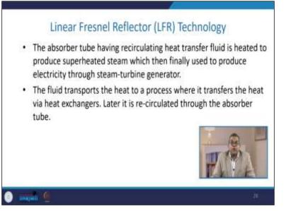
The absorber tube has the recirculating heat transfer fluid, which is heated to produce superheated steam, which is then used to produce electricity through steam turbine generators. The fluid transports the heat to a process where it transfers the heat via heat exchangers, and later it is recirculated through the absorber tube. The modified LFR system allows water to act as a transfer fluid or heat transfer media.
