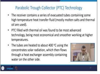
The receiver contains a series of evacuated tubes containing some high-temperature heat transfer fluid. This can be a molten salt, thermal oil, or synthetic oil. Depending on the use and how much heat transfer capacity you require, it can be used. These are filled with thermal oil, the most advanced technology, and the most economical and smoother working at high temperatures.
