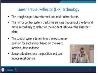
So, this trough surface is transformed into a multi mirror facet. The mirror control system tracks the sun rays throughout the day and moves according to the reflection accordingly
