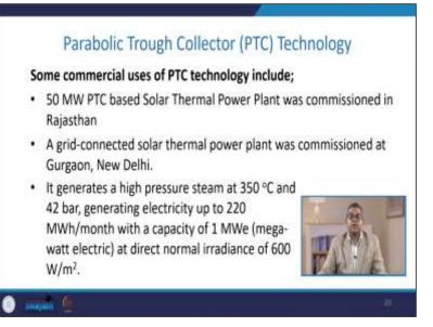
There are some commercial uses of the PTC technology, including the 50 megawatts PTCbased solar thermal power plant commissioned in Rajasthan. A grid-connected solar thermal power plant was commissioned at Gurgaon, New Delhi. Usually generates highpressure steam at 350 degrees Celsius and 42 bar, and it can generate electricity up to 220 megawatts with a capacity of one megawatt electric at direct normal irradiation of 600 watts per meter square.
