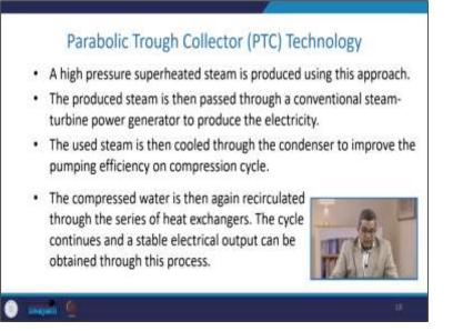
The compressed water is then again recirculated through the heat exchanger series, and the cycle continues and stable electrical output can be obtained through this process.
