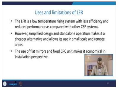
There are certain specific uses and apart from this limitation of LFR. This LFR is a lowtemperature rising system with less efficiency and reduced performance as compared to other CSP systems. Simplified design and standalone operation make it a good candidate because it is a cheaper alternative and allows its use in small-scale and remote areas. The use of flat mirrors and fixed CPC units make it more economical from the installation perspective. So, it is economically feasible in this respect.
