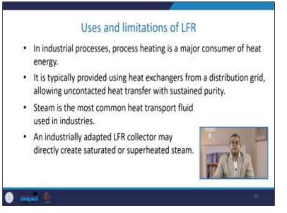
Industrial processes process heating is usually a major consumer of heat energy usually are typically provided using heat exchangers from a distribution grid, allowing uncontacted heat transfer with sustained purity. Steam is the most common heat transport fluid used in this particular industry. The industrially adopted LFR collector many directly created create saturated or superheated steam, and thereby it can be used in the steam power generation plant.
