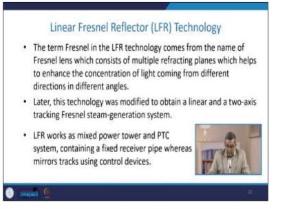
Later on, this technology was modified to obtain a linear and two-axis tracking of the fresnel system, which helped the steam generation system. This LFR works as a mixed power tower and PTC system containing a fixed receiver pipe whereas mirror tracks use control devices.
