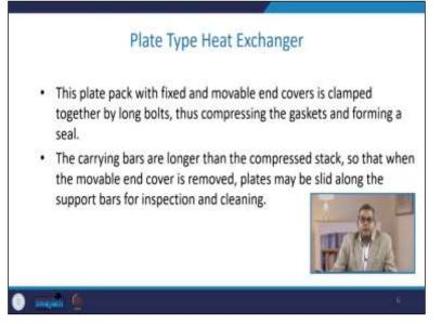
These plate packs with fixed and movable covers. Here you see that the fixed and movable covers are clamped together by a long bolt. Here you see that this is the long tightening bolt, thus compressing the gasket and forming a seal. So, the fluid or whatever the liquid or any kind of heat transfer material should not get leaked. Carrying bars are longer than the compressed stake. So, when the movable end cover is removed, the plate may be slid along the support bar for inspection and cleaning.
