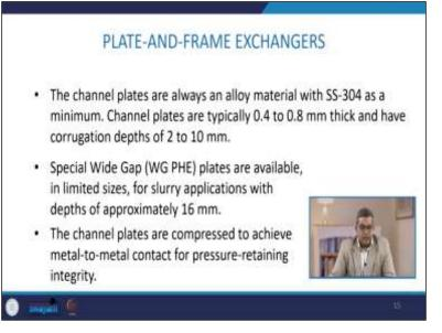
The channel plates are always an alloy material with the SS304 as a minimum. These channel plates are typically 0.4 to 0.8 millimeters in thickness and have a corrugation depth of 2 to 10 millimeters. Special wide gap WG PHE plates or plate heat exchangers are available in limited sizes for slurry application with a depth of approximately 16 millimeters. Usually, these channel plates are compressed to achieve metal-to-metal contact for pressure-retaining integrity.
