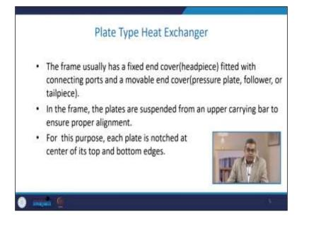
In the frame, the plates are suspended from an upper carrying bar. This is the upper carrying bar to ensure proper alignments. For this purpose, each plate is notched at the center of its top and bottom edge here you can see.
