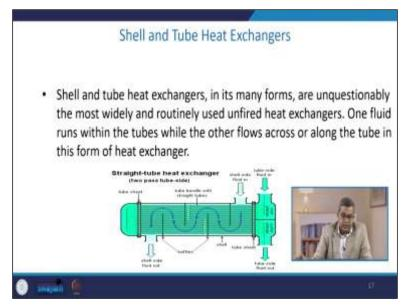
In its many forms, the shell and tube heat exchanger is unquestionably the most popular, most widely, or routinely used unfired heat exchanger. One fluid runs within the tubes while the other flows across the tube in the form of a heat exchanger. Now here, you can see there are two fluids one is the tube side fluid, and this is the shell side fluid. So, this is why because it offers the wide spectrum of uses with the help of different baffles and a lot of choices etc.
