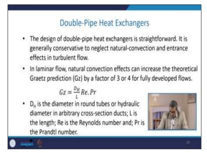
Now let us talk about the double pipe heat exchanger. The design of a double pipe heat exchanger is extremely straightforward. It is generally conservative to neglect the natural convection and entrance effect in a turbulent flow. The natural convection effect in laminar flow can increase the theoretical grades prediction G z by a factor of three or four for fully developed flows.
