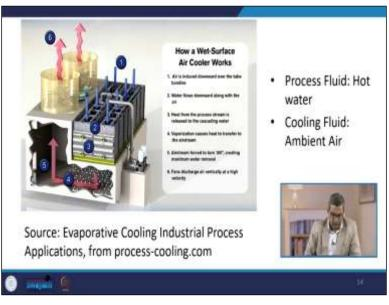
This is an example of evaporating cooling of industrial processes and applications. So, sometimes people may ask how a wet surface air cooler works. So, some of the air is induced downward over the tube bundles, water flows downward along with the air, and the heat from the process stream is released to the cascading water to the cascading water. Now the vapourization causes the heat transfer to the air stream.
