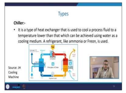
Now there are chillers. Now, this type of heat exchanger is sometimes used to cool a process fluid to a temperature lower than that, which can be achieved using water as a cooling media. And in this particular operation, a refrigerant like sometimes ammonia or a freon is used. So, this is the simplest form of a chiller here, you have a refrigerant, and this is the heat exchanger supplied with the cold water, which is where you require, say at a lower temperature.
