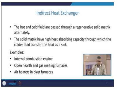
Examples of these indirect heat exchangers are internal combustion engines open earth, and gas melting furnace heat air heaters in the blast furnace.
