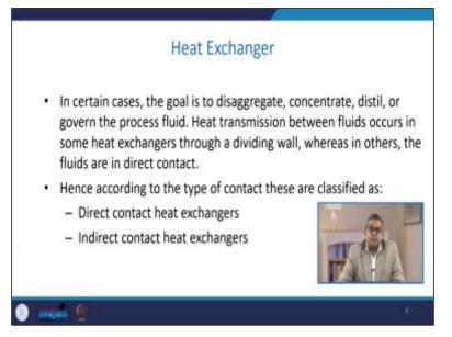
In certain cases, the goal is to disaggregate concentrate distillation performance; these govern the process fluid. Now heat transmission between fluids occurs in some heat exchangers; sometimes, the fluids are in direct, intimate contact through a dividing wall. So, when we talk about these two aspects, the heat exchangers can be classified in two ways: direct contact heat exchangers or indirect contact heat exchangers.
