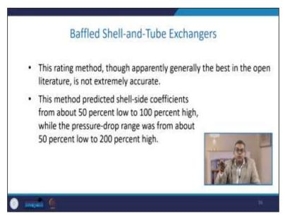
Though apparently the best in the open literature, this rating method is not extremely accurate. So while designing a very complex situation, you need some sort of accuracy.
