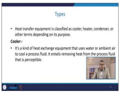
Now, when we; talk about the different types; so the heat transfer equipment is classified as a cooler heater condenser or other term depending upon its purpose and application. Now cooler is a kind of heat exchange equipment that uses water or ambient air to cool a process fluid. The other parameters can be fixed according to the requirement. Now it entails removing the heat from the process fluid that is perceptible.
