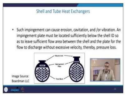
Now such impingement can cause erosion cavitation or vibration. An impingement plate must be located sufficiently below the shell's inner diameter to leave sufficient flow between the shell and the plate for the flow to discharge without excessive velocity and thereby pressure loss. Now here you see that these are the impingement plates, the nozzle and inlet, and the front section of the shell and tube heat exchanger. So, this is the tube bank.
