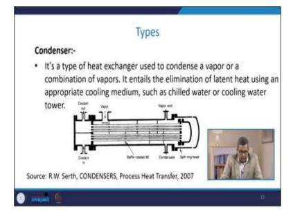
Now let us take a condenser, the most common type of thing being used in various chemical industries. Now, this is the type of exchanger used to condense a vapor, or a combination of different vapors may occur in any kind of chemical process. Now it entails the elimination of latent heat using an appropriate cooling medium, maybe sometimes chilled water cooling water or sometimes any kind of synthetic fluid which can be used or which can extract the desired quantum of heat from the fluid.
