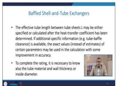
The effective tube length between the tube sheets L may be either specified or calculated after the heat transfer coefficient has been determined. Now, if additional specific information sometimes, like tube buffer clearance etc., is available, the exact value instead of the estimated or assumed value of certain parameters may be used in the calculation of some of the improvements in the calculation with some accuracy.
