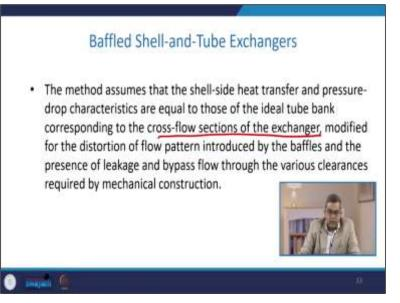
The method assumes that shell side heat transfer and pressure drop characteristics are equal to those of the ideal tube bank that corresponds to the cross-flow section of the exchanger, modified for the distortion of the fluid pattern introduced by the baffle and the presence of leakage and bypass flow through the various type of a clearance they require the by the as required by the mechanical construction.
