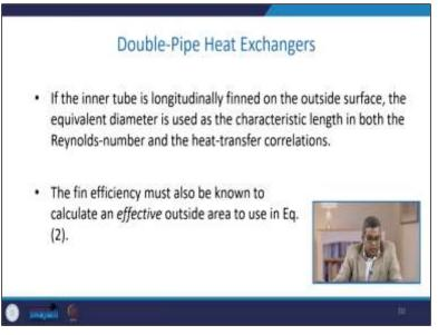
If the inner tube is longitudinally finned on the outside surface, the equivalent diameter is used as the characteristic length in both the Reynolds number and the heat transfer correlation. So, the fin efficiency must also be known to calculate an effective outside area to use in the previous equation.
