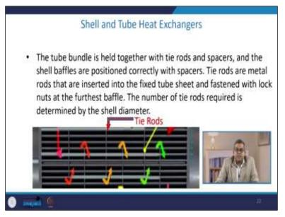
And spacers, the shell baffles are positioned correctly with a spacer. Now tie rods are metal rods that are inserted into the fixed tube sheets and fastened with the lock nuts at the furthest level. The number of tie rods required is determined by the shell diameter what is the shell diameter. So, based on this one, you can assess how many tie rods are required. (**Refer Slide Time: 20:19**)
