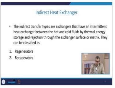
The indirect heat transfer type is the heat exchangers with intermittent heat exchange between the hot and cold fluids by thermal energy, which may be by storage rejection through the exchanger surface or matrix. Now they can be further classified as regenerators or recuperators. The hot and cold fluid are passed through a solid regenerative matrix alternately. The solid matrix has a high heat-absorbing capacity through which the colder fluid transfers the heat as a sink.
