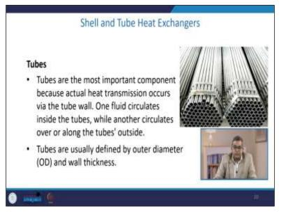
Tubes are the most important component because actual heat transmission or heat transfer occurs via the tube wall. Here you can see the bundle of tubes. One fluid circulates inside
