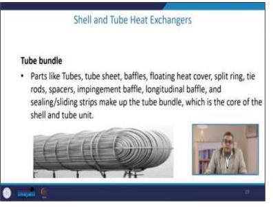
The tube bundle is again the integral part of the SNT or shell, and tube heat exchanger like parts like tubes, tube sheets, baffles, floating heat cover, split ring, tie rods, spacers, infringement baffle, longitudinal baffle, sealing/sliding strips they make the tube bundle, you can see over here the tube bundle which is the core or you can see the heart of any shell and tube heat exchanger.
