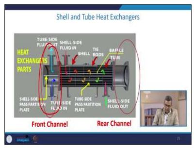
Now here you see the concept of the front channel and the rear channel. Now, this is the shell side pass partition plate, and here you see the shell fluid in, and here the tube side fluid in. This is the tube side pass partition plate shown.
