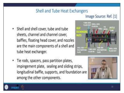
Now shell and shell cover tube and tube sheets channels and channel cover baffles floating head cover nozzles they are the main component of any type of a shell and tube heat exchanger you can see here this is again the anatomy of shell and tube heat exchanger. Now tie rods spacers pass partition plates impingement plates ceiling and sliding strips longitudinal baffle supports and foundation are among the other components which are required in the shell into the heat exchanger.
