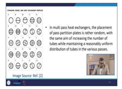
Now there are various standard vessel and heat exchanger profiles. So, in the multipass heat exchanger, the placement of pass partition plate is rather random to increase the number of tubes while maintaining a reasonably uniform distribution of tubes in various passes.
