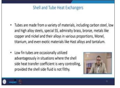
Tubes are made from a variety of materials, including carbon steel, low and high alloy steel, a special type of stainless steel, admiralty brass, bronze, metal like copper and nickel, and their alloys in various proportions, monel, titanium, and even exotic material like hast alloys and tantalum. Low fin tubes are sometimes utilized advantageously when the shell side heat transfer coefficient is very controlling, provided the shell side flute is not flitty.
