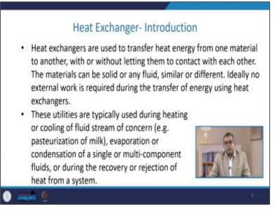
So, the basic concept of heat exchangers is that they are used to transfer the heat energy from one source to another without letting them contact each other. So, this is again a very crucial aspect. Sometimes, you need to let the intimate contact between the heat transfer media and the process material be in question, or sometimes you do not. These materials can be solid or any fluid similar or different ideally. No external work is required to transfer energy using a heat exchanger.
