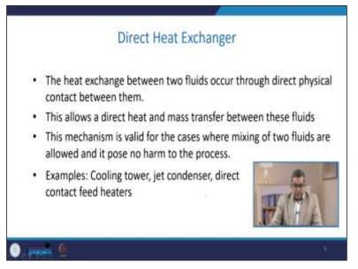
Now let us have a brief outlook on the direct heat exchanger or direct type of heat exchanger. Now the heat exchange between two fluids occurs through direct physical contact between them. Now, this allows a direct heat and mass transfer between these two fluids because they are in direct contact; then again, the mass transfer will occur. Now, this mechanism is valid for the cases where mixing two fluids is allowed and poses no harm to the process.
