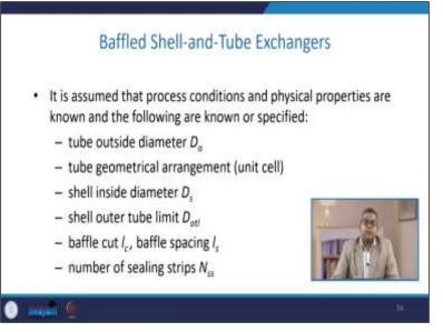
It is assumed that the process conditions and physical properties are known, and different types of parameters that should also be known are enlisted, like tube outside diameter  $D_o$ . Then tube geometrical arrangement per unit cell then shell inside diameter  $D_s$ , shell outer tube limit, baffle cut, baffle spacing, and number of ceiling strips referred as  $N_{ss}$ .
