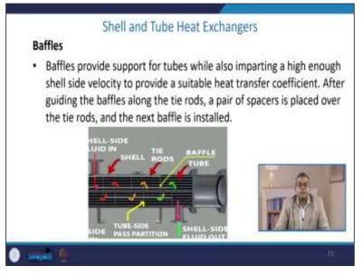
Then baffles provide support for the tubes while imparting a high enough shell side velocity to provide a suitable heat transfer coefficient. After guiding the baffles along the tie rods, a pair of a spacer is placed over the tie rods, and the next baffle is installed. So, you can see these are the tie rods these are the baffle tubes.
