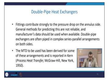
Now fitting use usually contributes strongly to the pressure drop on the annulus side. Now a general method for predicting this is for this usually they are not reliable and manufacturers data should be used when available and usually all the manufacturers they use to supply such kind of calibration data. Now double-pipe exchangers are often piped in complex series-parallel arrangements on both sides.
