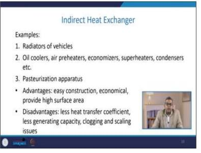
Let us have a couple of examples like the radiator of vehicle oil coolers, air preheaters, economizers, superheaters, being used in different types of boilers, condensers,
