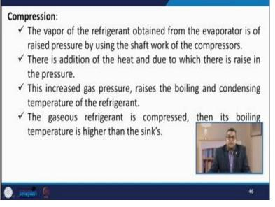
Now let us talk about the compression. The Vapour of the refrigerant is obtained from the evaporator is of raise the pressure by using the shaft work of the compressor. Now there is addition of heat and due to which there is a raise in the pressure because the compressor the work is employed on the compression. Now, this increased gas pressure rises in the boiling and condensing temperature of the refrigerant.
