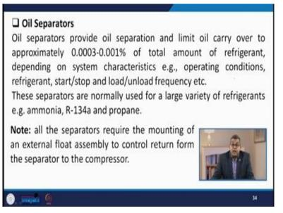
Then there are certain oil separators and they are used to remove oil in due course of time because during the circulation refrigerant may accumulate some some sort of traces of oil and these oil needs to be separated from the main refrigerant to make the system more and more efficient. So this these oil separators they provide the oil separation and limit oil carry over to approximately 0.0003 to 0.001% of total amount of refrigerant.
