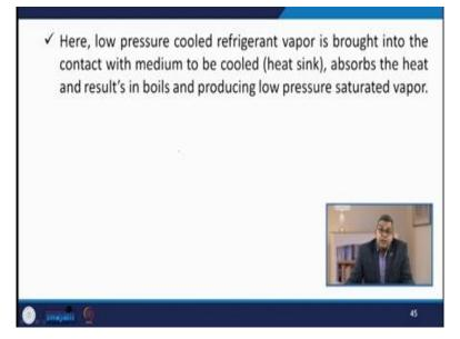
So the low-pressure cooled refrigerant vapour is brought into the contact with the medium to be cooled and that is called the heat sink and absorbs the heat and results in boil and producing low pressure saturated vapour.
