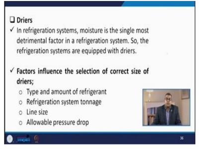
Basically we are dealing with the quantity and the quality then refrigeration, system with respect to the tonnage then the line size and allowable pressure drop.
