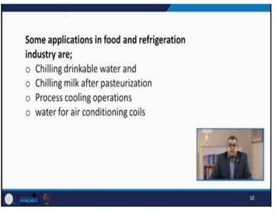
Now, there are some applications in food and refrigeration industries like chilling drinkable water, chilling milk after pasteurization. It can be used for refrigeration system in the process cooling operation then water for the air conditioning coils.
