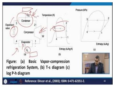
Now here you see this is the comprehensive figure here you are. This is the usual refrigeration cycle. You are having a low temperature source and a high temperature sink. So Q L amount of heat is being extracted through the evaporator and it passes through the compressor and it goes to the condenser where the Q H amount of heat being discharged either to the atmosphere or sink and goes to the expansion valve.
