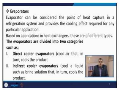
Now let us talk about the evaporators. Now evaporator, this can be considered the point of heat capture in refrigeration system and provide the cooling effect required for any particular application. Now based on applications in heat exchanger there are different types of evaporators. So the evaporator when we are talking about a different type of evaporators then again there may be a need of a classification or categories so the evaporators they are basically divided into 2 categories.
