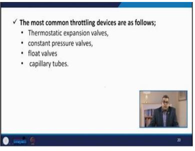
There are various kinds of throttling devices. The most common throttling devices are the thermostatic expansion valves the constant pressure valves, float valves and the capillary tubes.
