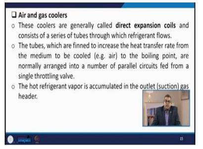
Now these coolers are generally called the the direct expansion coils and consists of a series of tubes through which refrigerant flows. The tubes which have finned to increase the heat transfer
