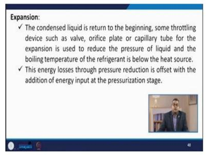
Now this energy loss through a pressure reduction is offset with the addition of energy input in the pressurization stage.
