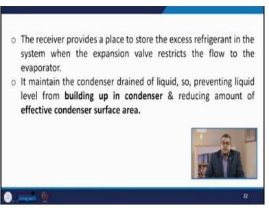
Now this the receiver they provide a place to store the excess refrigerant in the system when the expansion valve restricts the flow to the evaporator it usually maintain the condenser drained of liquid. So preventing liquid level from building up in condenser and reducing amount of effective condenser surface area.
