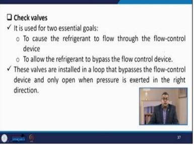
Next is a check valve now it is used for 2 basic essential goals. One is to cause the refrigerant to flow through the flow control device and second is to allow the refrigerant to bypass the flow control device. Now these valves are installed in a loop that bypasses the flow control device and only upon when pressure is exerted in the right direction.
