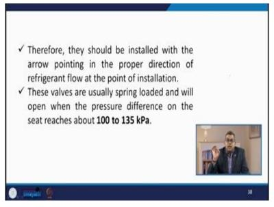
So therefore they should be installed with the arrow pointing in the proper direction of the refrigerant room, at the point of installation. Now, these valves are usually spring loaded and opens when the pressure difference on the seat reaches around about 100 to say 135 kilo Pascal. (**Refer SlideTime: 23:03**)
