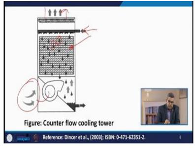
Here you see here the air is circulating through this one and this is the packing, the mesh size you can see and these are the droplets and here the water is circulated and this is the exhaust air outlet.
