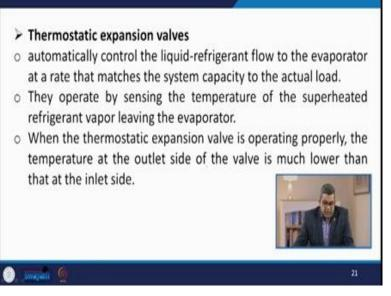
Now let us talk about the thermostatic expansion valves. Now they are basically automatic type so automatically control the liquid refrigerant flow to the evaporator at a rate that matches the system capacity to the actual load. Now they operate by sensing the temperature of superheated refrigerant vapor leaving the evaporator. Now when the thermostatic expansion valve is operating properly the temperature at the outlet side of the valve is much lower than that at the inlet side.
