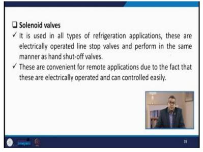
Solenoid valves now it is used in all type of refrigeration applications and these are electrically operated line stop valves and perform in same manner as hand shut off valves. Now these are convenient for remote application due to the fact that these are electrically operated and can control easily.
