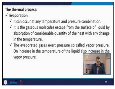
Now in a elaborative manner the evaporation process. It can occur at any temperature and the pressure combination. It is the gaseous molecule escape from the surface of liquid by the absorption of considerable quantity of heat with any change in the temperature. It is a usual phenomena of evaporation. The evaporated gases they exert pressure and that is so called the vapor pressure on increasing the temperature of the liquid this also increase the vapour pressure.
