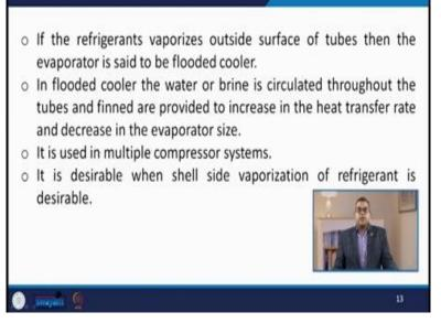
Now if the refrigerant vaporizes outside the surface of the tube, then the evaporator; is said to be called a flooded type of cooler now in flooded cooler the water or brine is circulated throughout the tubes and fins are provided to increase the heat transfer rate and decrease the evaporator size. Now, it is used in multiple compressor type of system. Now it is desirable when shell side, vaporization of refrigerant is desirable.
