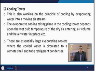
So let us talk about the cooling tower, although in a separate lecture we had deliberated or you can say the exhaustive discussion about the cooling towers but again in the refrigeration system, they are also integral part. So this is also working on principle of cooling by evaporating water into a moving air system. Now, this evaporative cooling it takes place in the cooling tower. It depends on the wet bulb temperature of the dry air entering air volume and the air water interface.
