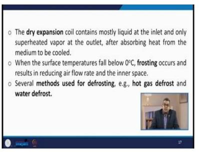
The dry expansion coil sometimes they contain mostly liquid in the inlet and only superheated vapour at the outlet and after absorbing heat from the medium to be cooled. When the surface
