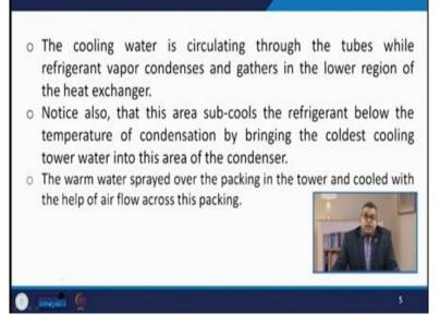
The cooling water is circulating through the tubes while refrigerant vapour condenses and gathers in the lower region of the heat exchanger. Now, this Particular area sub cools the refrigerant below the temperature of the condensation by bringing the coldest cooling tower water into this area of the condenser. Now the warm water is spread over the packing in the tower and cooled with the help of air flow across this particular packing.
