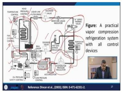
Now, here you see this is the practical vapor compression refrigeration system with all kind of control device and you see that how mammoth it is the task. Here you are having this evaporator with the equipped with the temperature control device and usually when we are talking about the evaporator it should be a series of thermo valves with the hot gas bypass regulator.
