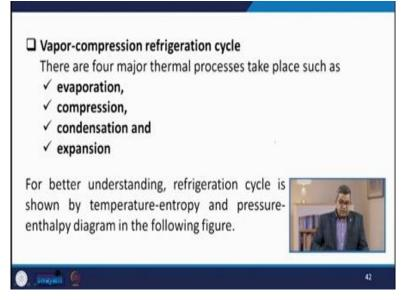
Now let us think about the vapour compression refrigeration cycle. Now there are 4 major steps or you can say that thermal processes. They usually carried out in the vapour compression refrigeration cycle. One is evaporation compression condensation and expansion. It is a usual thermodynamic cycle for better understanding the refrigeration cycle is usually shown by the temperature entropy or pressure enthalpy diagram.
