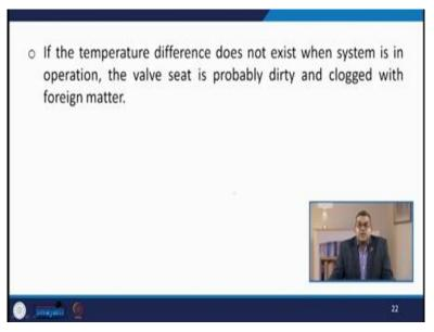
Now, if temperature difference does not exist, when the system is in operation the valve seat is probably dirty and clogged with foreign matter.
