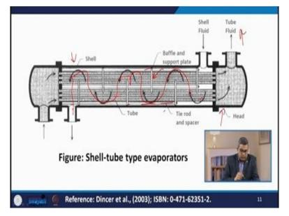
Now here you see that this is the typical photograph or figure of shell and tube, type of evaporators. Now, this is the shell and this is duly supported by baffles and support plates. And here, you see that this is the tube side fluid and head and these baffles are supported with the tie rods and this is the tube. So the shell side tube and you can see the circulating path of the fluid in this arena.
