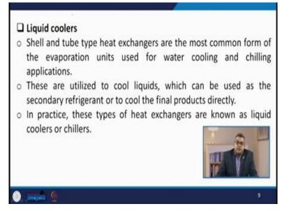
So let us talk about the liquid coolers. Now shell and tube type of heat exchangers. They are the most common form of evaporation units used for water cooling and chilling applications. Now, these are utilized to cool liquids which can be used as the secondary refrigerant or to cool the final product directly. So in practice, these types of heat exchangers they are known as liquid cooler or chillers.
