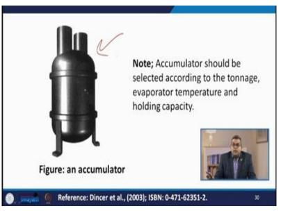
Now here you see this is the typical photograph of an accumulator. This accumulator should be selected according to the tonnage of refrigeration system, according to the evaporator temperature and according to the holding capacity.
