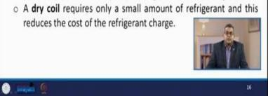
Now these direct expansion coils are sometimes used only in the positive displacement compressor type of a system owing a quite low pressure ratio. Now these are classified as the flooded and dry type in practical applications flooded type evaporators are not preferable because they required large amount of refrigerant. A dry coil requires only a small amount of refrigerant and this reduces the cost of refrigerant charges.
