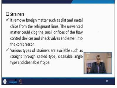
The unwanted matter they can clog the small orifice of the flow control device even the throttling device and check valves and enter into the compressor. Now the various types of strainers available as on date such as state through seal type, cleanable angle type and cleanable y type. Next is the dryer in refrigeration system moisture is the single most detrimental factor in the refrigeration system.
