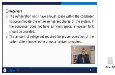
Now next is the receiver the refrigeration units that have enough space within the condenser to accommodate the entire refrigerant charge of the system. Now if the condenser does not have sufficient space a receiver a tank should be provided. The amount of refrigerant required for proper operation of the system this determines whether or not a receiver is required or required or not required.
