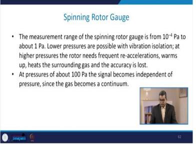
The measurement range of the spinning rotor gauge, is from 10 to the power -4 Pascal to about 1 Pascal lower pressure are possible with the vibration isolation at higher pressure. The rotor needs frequent re-acceleration, warms up heat and surrounding gas and accuracy is lost. At pressure of about say, 100 Pascal, the signal become independent of the pressure. Since the gas becomes continuum.
