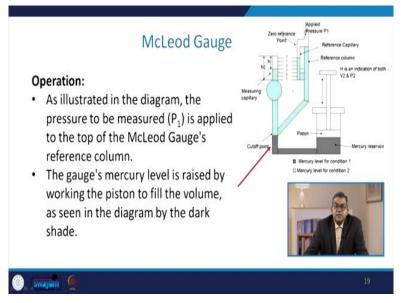
Now here you see, this is the piston. Now let us talk about the operation of this McLeod gauge now. This is very well illustrated in this particular figure. The pressure to be measured P 1 is applied at the top of McLeod gauge. Now here you see, now the gauge gates, mercury level is raised by the working, the pressure to fill the volume, as per the you can see in this particular figure.
