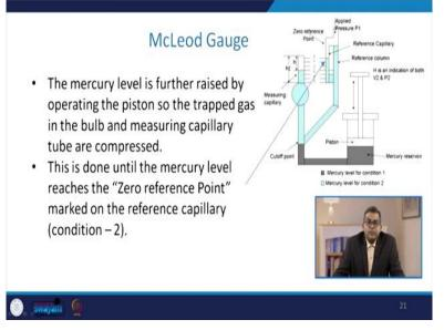
The mercury level is further raised by operating the piston, so, the trapped gas in the bulb and mercury capillary tubes are compressed. Now this is done until the mercury level reaches to the zero-reference point. Now here this is the zero-reference point now, in this condition, the volume of the gas in the measuring capillary tube is read directly by the scale beside it and that is the difference in the height delta h.
