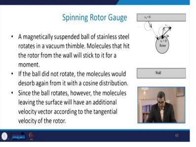
The magnetically suspended ball like this of steel rotates in a vacuum thimble. The molecules that hit the rotor from the wall will stick to it for a moment. Now if the bar did not rotate, the molecules would dissolve again from it with a cosine distribution. Now, since the ball rotates, however, the molecule leaving the surface will have an additional velocity vector according to the tangential velocity of the rotor.
