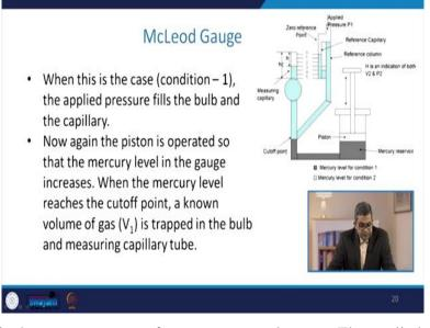
Now, when this is the case, you can refer as a case number one. The applied pressure fills the bulb and the capillary. Now again, the piston is operated so, that the mercury level in the gauge increases when the mercury level reaches the cutoff point known volume of gas. That is sometimes referred as V 1 is trapped in the bulb and measuring the capillary tube.
