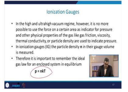
Now in the high and ultrahigh vacuum regime. However, it is no more possible to use the force on a certain area as indicator for the pressure and other physical proportion of the gas like gas friction, viscosity, thermal conductivity or particle density they are used to indicate the pressure. Now in ionization gauges the particle density n in the gauge volume is measured. Therefore, it is important to remember the ideal gas law for enclosed system in equilibrium that is p is equal to n k T.
