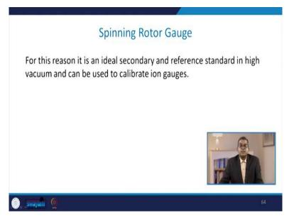
Now, for this reason it is an ideal secondary reference standard in high vacuum and can be used to calibrate ion gauges.
