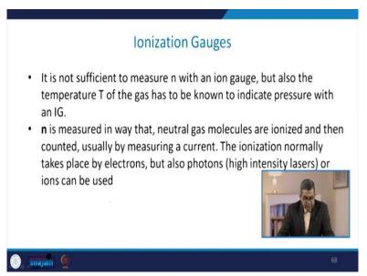
It is not sufficient to measure n with an iron gauge, but also the temperature T of the gas has to be known to indicate pressure with an IG. Now n is measured in a way that the neutral gas molecules are ionized and then counted usually by measuring a current. The ionization normally takes place by electron, but also photon that is a high intensity laser or ions can be used.
