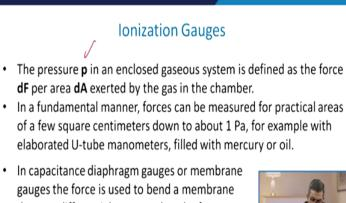
In capacitance diaphragin gauges of membrane gauges the force is used to bend a membrane due to a differential pressure, but the force cannot be determined in a fundamental way and the gauge has to be calibrated.
