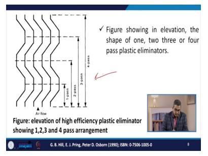
Now, this particular figure shows the in elevation, the shape of 1, 2, 3 or 4 pass the plastic eliminator. Now here you see that this is the one pass and this is the two pass and a three pass and a four-pass type 1, 2, 3, 4 pass type of eliminator
