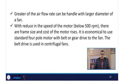
Now, with the reduce reduction in the speed of the motor below say 500 rpm there are frame size and the cost of the motor rises. So, you have to look into this while optimizing the appropriate fan. Now, it is economical to use the standard 4 pole motor with belt or gear drive to the fan and the belt drive is used in the centrifugal fan.
