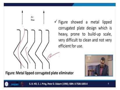
Now here this particular figure representing a metal lipped corrugated plate design which is heavy, prone to build-up scale and very difficult to clean and not very efficient for use now this is you see this is the metal lipped corrugated plate eliminator
