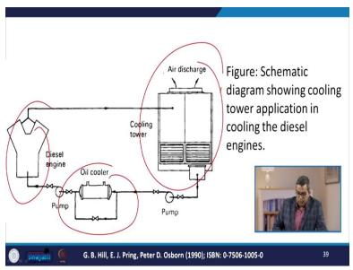
Now, here this is the diesel engine and with the help of this oil cooler it can be removed with the help of this cooling tower.
