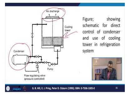
Now, here you see that the schematic diagram for direct control condenser and use of cooling tower in the refrigeration system. Now, here you see this is the condenser and air discharge assembly and rest other things are common which we have already discussed in the previous lectures.
