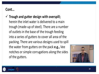
Now trough and gutter design over with overspill. Now, this is in this particular type of system the inlet water is delivered to a main trough that is usually made up of steel and there are a number of outlets in the base of the trough feeding into a series of gutters to cover all area of the packing.
