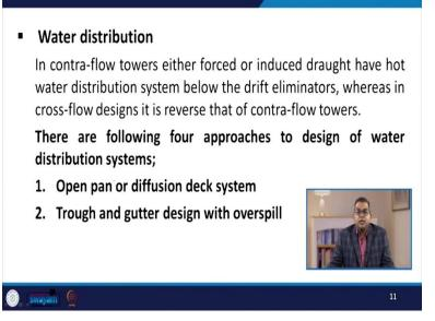
Whereas in cross flow design it is reversed that of the contraflow towers there are four approaches of design of water distribution system. Now one is open pan or diffusion deck system. Second, is the trough and gutter type of design with overspill.
