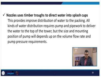
Now, nozzles they uses use the timber trough to direct water into splash cups now this provides improved distribution of water to the packing. Because improved distribution of water in the packing is quite essential for the proper efficiency of the cooling tower as well as it imparts the energy efficiency aspect too. So, the cost of running of the cooling tower may be lower down.
