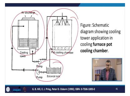
Now here you see that this cooling tower is same, but this is the pre-cooling chamber and this is the balance tank. This is a stigmatic diagram, showing the cooling tower application for the furnace spot cooling chamber.
