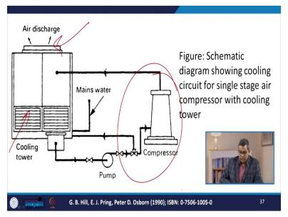
Now, here you see that this is the schematic diagram for showing the cooling circuit for single stage air compressor. Now here you see, this is the single stage air compressor and rest other things like packing air discharge. All these things as usual which we have discussed earlier
