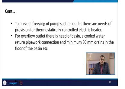
For overflow outlet there is need of basin a cold-water return, pipe work connection and a minimum 80 mm drain in the floor of basin.
