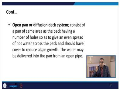
Now, let us talk about the open pan or diffusion deck system usually consists of a pan of same area as pack having a number of holes. So, as to give an even spread of hot water across the pack and should have covered to reduce algae growth because algae grow sometimes it creates a massive problem and the water may be delivered into the pan from an open pipe.
