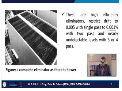
Now, these types of eliminators are highly efficient and they restrict the drift to 0.005, with the single pass of to 0.001% with two pass and nearly undetectable levels with the three to four passes. (**Refer Slide Time: 05:49**)
