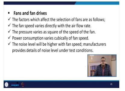
Now, fans and fan drive as we were discussing in the previous lectures. They are again the integral part of the cooling tower the factors which affect the selection of fans they are quite complicated and we need to address for the proper efficiency of this cooling tower. So, there are various factors associated with such kind of selection criteria one is that the fan speed varies directly with the air flow rate.
