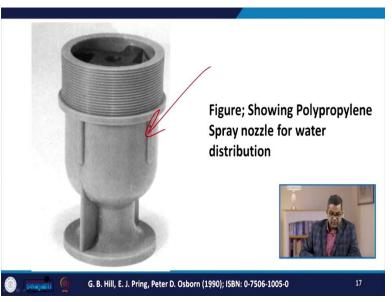
Now, this is the figure which shows the polypropylene spray nozzle for water distribution.
