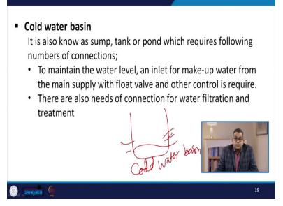
Now, if you recall that at the bottom of the cooling tower there is a cold-water basin. Now, this is sometimes known as a sump, tank or pond which requires different type of connections. Now, one is to maintain the water level because appropriate water level is essential and that is why the walls or the floating walls are there and inlet to make up water from the main supply with the float wall and other control which is required.
