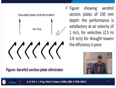
Now, this particular figure shows the aerofoil section plate eliminator. Now this aerofoil section plate of 150-millimeter depth. The performance is satisfactory at air velocity of 1 meter per second for velocities, ranging from 2.5 to 3 meter per second for draught tower. Now the efficiency is extremely poor in this particular type of air force section of eliminator.
