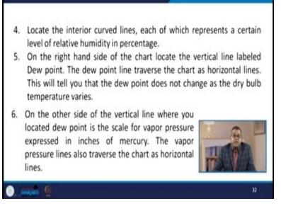
Now locate the interior curve lines here you need to locate the interior curve lines of which represent a certain level of relative humidity in percentage. Now on the right hand side of the chart, locate the vertical lines labeled as a dew point. The dew point of the line traverse the chart as horizontal line and this will let you know the dew point does not change as the dry bulb temperature varies.
