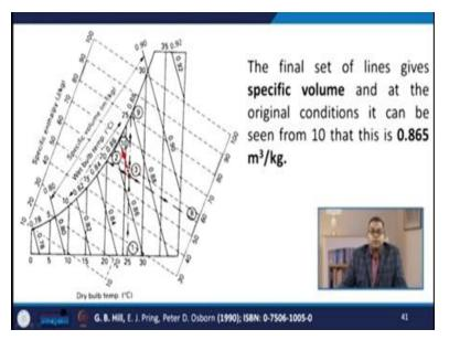
The final set of lines, this gives the specific volume and the original condition can be assessed and that is 0.865 meter cube per kilogram.
