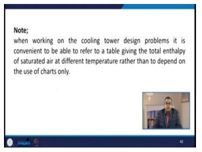
Now when, working on the cooling tower design problem it is convenient to able to refer to a table giving the total enthalpy of saturated line air at different temperature rather than to depend on the use of charts only. Now when; we talk about the wet bulb temperature and the system equilibrium. Suppose that the unsaturated air is brought into contact with the liquid water under adiabatic condition there is no heat transfer take place between the systems.
