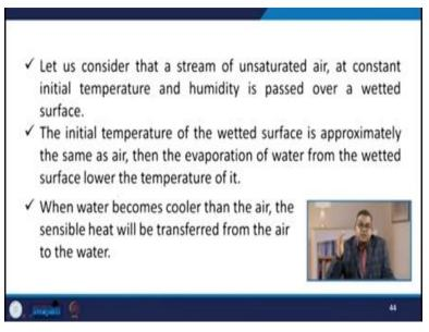
Now when, water become cooler then air the sensible heat will be transferred from air to water.
