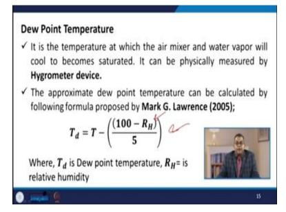
Another important point which we need to address and that is the dew point temperature. It is a temperature at which the air mixture and water vapor will cool to become the saturated. It can be physically measured by hydrometer device. The approximate dew point temperature can be calculated by this particular mathematical relationship given by Lawrence and that is equal to  $T_d = T - 100 - R_H$  upon 5. Now  $T_d$  is the dew point temperature and  $R_H$  is the relative humidity.
