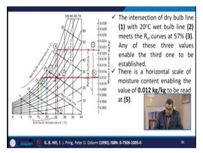
And that is the most practical approach. Now here you need to find out first the intersection of dry bulb line. Now here you see that this is the dry bulb line. This is the dry bulb temperature here the wet bulb temperature curve and this relative humidity. So this intersection of dry bulb line with say 20 degree Celsius here you see this is a 20 degree Celsius meets the relative humidity curve.
