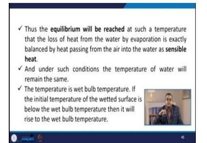
Thus, the equilibrium will be reached at such temperature and that the loss of heat from water by evaporation is exactly balanced by the heat passing from air into the water as sensible heat. Now under such conditions the temperature of water will remain the same. The temperature is the wet bulb temperature, and if the initial temperature of the wetted surface is below the wet bulb temperature. Then it will rise to the wet bulb temperature.
