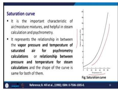
Now sometimes in different engineering perspective, you need to look bout the saturation curve. Now it is the important characteristic of air moisture mixture and it is helpful in steam calculation and psychrometric. It represents a relationship in between the vapor pressure and the temperature of saturated air for psychrometric calculation or relationship between the pressure and temperature for steam calculations.
