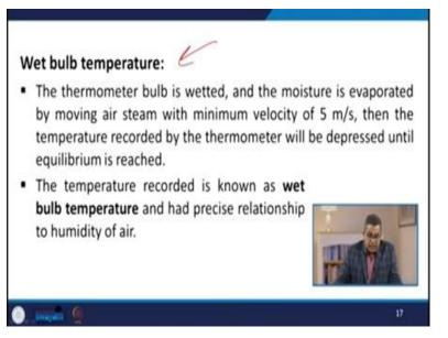
Another important thing that is called up wet bulb temperature. Thermometer bulb is wetted and the moisture is evaporated by moving air steam with the minimum velocity of say 5 meter per second. Then the temperature recorded by the thermometer will be depressed until equilibrium is reached. So, whatever temperature is recorded, that is known as a wet bulb temperature and had precise relationship to humidity of air.
