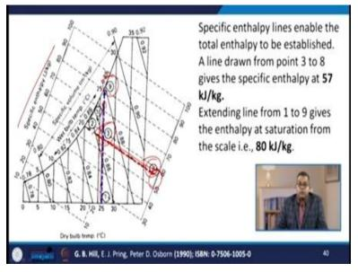
Now specific enthalpy lines these enable the total enthalpy to be established. Now if we draw a line from point number 3 to 8 like this gives the specific enthalpy that is 57 kilogram per kilo joule. Now if we extend this line further to the point number 9 here. It gives the enthalpy at saturation from the scale and this comes out to be nearly 80 kilo joule per kilogram.
