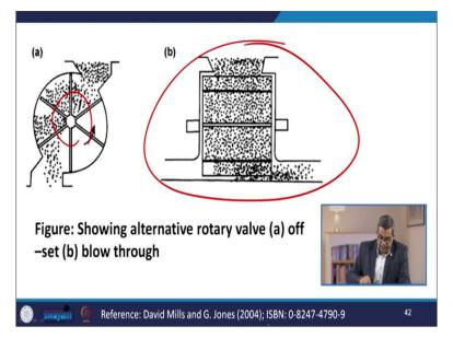
Now here you can see the figure which we were referring about. The rotor movement is just like this and this is the typical anatomy of the subsection of this rotary valve. Now, this is the off-set and this is the blow through.
