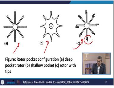
Now you see different type of rotor pocket configuration. This is the deep pocket rotor, shallow pocket and rotor with tips here you see the different tips.
