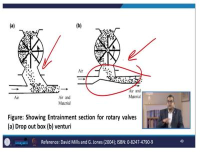
Now here you see that the entrainment section of rotary valves. Now here this is the drop out box and this is the Venturi and rest other function is common.
