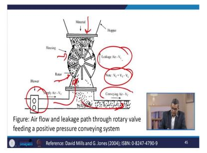
Now here you see we are feeding the material and material is coming out from here. This is subjected to the rotor and housing as depicted previously with the help of blower you are supplying the air to the system. Now, if we consider the leakage of air that is V L so V C = V S - V L where V C is the conveying air.
