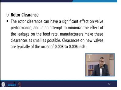
Now next is the rotor clearance. The rotor clearance can have a significant effect on valve performance and in attempt to minimize the effect of the leakage on the feed rate. Manufactures may make these clearances as small as possible. Now clearances on new valves they are typically in the order of 0.003 to 0.006 inches.
