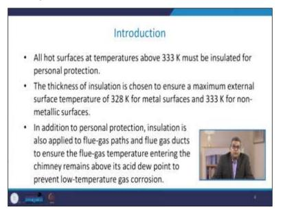
When we talk about insulation, all hot surfaces at a temperature above 333 Kelvin must be insulated for personal protection. It not only ensures the personal safety or the person those who are working around that particular surface must be safe but also ensures that the system's thermal efficiency must be secured properly. The thickness of insulation is usually chosen to ensure a
