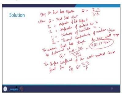
Now we have we can use the heat loss equation Q is equal to T h - T c upon L by k where Q is equal to heat loss in watt per meter square T h is equal to temperature of hot surface Kelvin T c is the temperature of ambient air in Kelvin L is the thickness of insulation in meter k is the thermal conductivity of insulator in watt per meter Kelvin.
