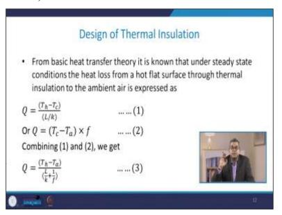
Now let us talk about the design of thermal insulation. From basic heat transfer theory, it is known that under steady-state conditions, the heat loss from a hot splat surface through thermal insulation to the ambient air is usually expressed as
