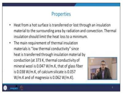
Let us talk about the properties. Now heat from a hot surface is transferred or lost through an insulating material to the surrounding area either by radiation or by convection. Thermal insulation should limit heat loss to a minimum. One main requirement of thermal insulation material is low thermal conductivity since heat is transferred through insulating material by conduction at 373 Kelvin thermal conductivity of said mineral.
