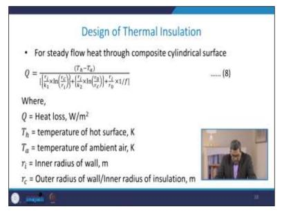
For steady flow heat through composite cylindrical surface
