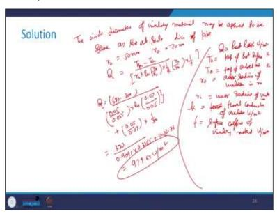
The inside diameter of insulating material may be assumed to be the same as the outside diameter of the pipe.
