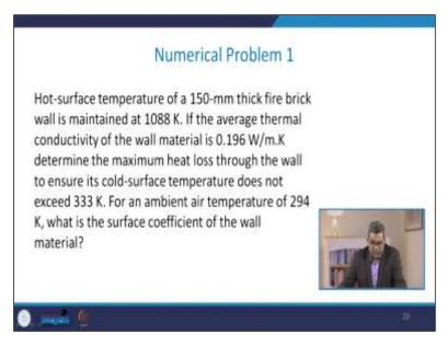
Now let us talk about couple of numericals problem. Now for problem number one the hot surface temperature of 150 millimeter thick fire brick valve is maintained at 1088 Kelvin. Now if the average thermal conductivity of the valve material is 0.196 watt per meter Kelvin you need to determine the maximum heat loss through the valve to ensure its cold surface temperature does not exceed 333 Kelvin.
