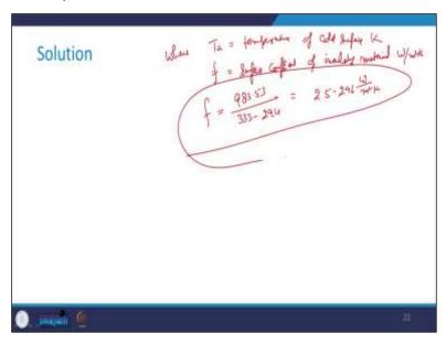
The surface coefficient of the wall material can be found from Eq. 2 as
