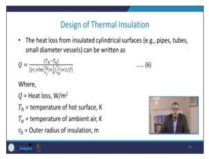
The heat loss from insulated cylindrical surfaces (e.g., pipes, tubes, small diameter vessels) can be written as
