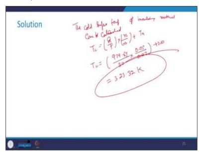
The cold surface temperature of the insulating material can be calculated using eq. 7as,
