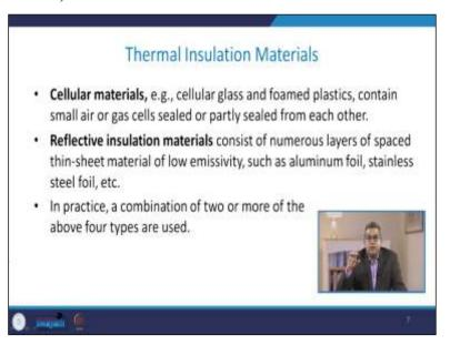
Now the third category is the cellular materials which are cellular glass and foam plastics. This contains small air or gas cells sealed or partly sealed from each other. These are reflective insulation materials. This consists of numerous layers of spaced thin sheet metal materials with
