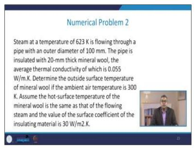
Now steam at a temperature of 623 Kelvin is flowing through a pipe with an outer diameter of 100 millimeter the pipe is insulated with 20 millimeter thick mineral wool the average thermal conductivity of which is 0.055 watt per meter Kelvin. You need to determine the outside surface temperature of mineral wool if ambient temperature is 300 Kelvin. You may assume the hot surface temperature of the mineral wool is the same as that of the flowing steam.
