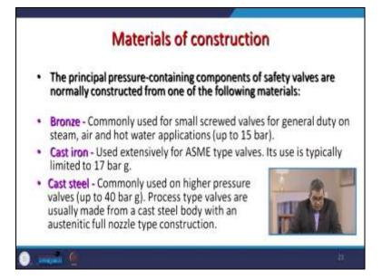
The principal pressure-containing components of safety valves are normally constructed from different metal materials like bronze is commonly used for a small screwed valve for general duty in steam air and hot water application that may be used up to 15 bar. Cast iron is usually used extensively for ASME (American Society For Mechanical Engineering) type of valve have designed their own codes.
