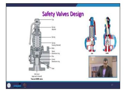
This is the anatomy of the safety valve. You see that this is the cap and this is the spring adjuster to meet any kind of a fluctuation within the system. This is the spring, and based on the spring constant this usually works; and this is spring housed in a system that is called the bonnet, through which a protective shell can be designed. This is the main body, and this here you see this is the blowdown ring and this is the main thing that is the disc, and this is the seat.
