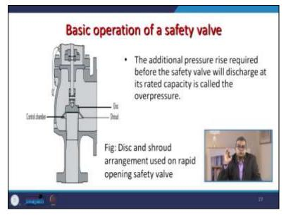
The additional pressure riser here you see that is a more closer look this is the disc, and this is the seat. the additional pressure rise required before the safety valve will discharge at the rate its rated capacity is called overpressure.
