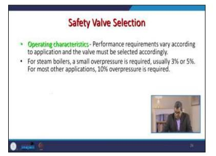
Another foremost criterion for the safety valve selection is the operating characteristics. Performance requirements may vary according to application, and the valve must be selected accordingly. For steam boilers, a small overpressure is usually required, say 3 to 5% for most of the replication 10% overpressure. A very important part of safety valve selection is the approval.
