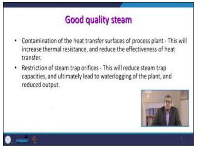
So, if there is a restriction in the steam trap orifice this will reduce the steam trap capacity and ultimately lead to the waterlogging of the plant and reduce the output.
