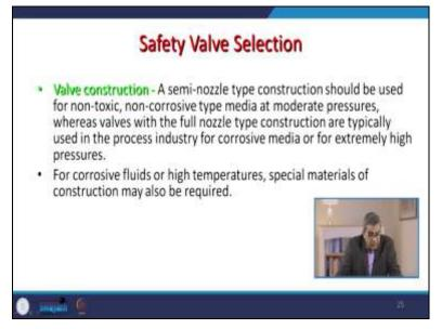
Then the valve construction is a semi-nozzle type construction. This should be used for nontoxic, non-corrosive type media at moderate pressures. At the same time, evolved with the full nozzle type construction is typically used in the process industry for corrosive media or for extremely high pressure. So, if we are using corrosive fluid or high-temperature special construction material, this may also be required.
