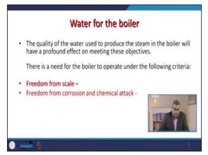
These criteria include that it must have freedom from scale and freedom from corrosion, and chemical attack. In the previous lectures, we discussed the concept of scale, how these scales are
