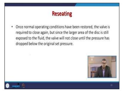
Next is the reseating because once you restore the normal operation condition, the valve is required to be close again. Since the large area of the disc is still exposed to the fluid, the valve will not close until the pressure has dropped below the original set pressure. So, you have to look at this particular equilibrium between the disk and the boiler pressure.
