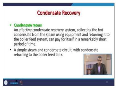
When we talk about the condensate return and an effective condensate recovery system usually collects the hot condensate from the steam using the equipment and returns it to the boiler feed system and can pay itself for a remarkably short period of time because the heat value as well as the water value always very you can say the attractive things in the condensate recovery. A simple steam and condensate circuit must be properly designed with the condensate returning to the boiler tank.
