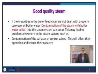
So, for good quality of steam, the impurities in the boiler feed water are not appropriately dealt then the carryover of a boiler means the contamination of the steam with boiler water solids into the steam system can occur. And this may lead to a problem elsewhere in the steam system. As I discussed, if you are directly introducing steam, this steam into any chemical reaction even the small metal particles may participate in the reaction.
