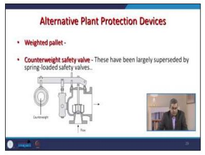
Another thing is that weighted pallets, and previously various boilers are using the counterweight safety valves. The spring loaded safety valves largely supersede these. here, the concept is common you have weights, and this is the steam generation unit or boiler. If and this particular seating or reseating arrangement is usually complemented or supplemented by these counterweights.
