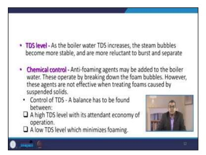
The TDS level as the boiler water TDS increases, the steam bubbles become more stable and more reluctant to burst and separate. There are certain chemical controls like adding certain anti-foaming agents or chemicals that may be added to the boiler water. This operates by breaking down the foam bubbles, which means are the surface active agents. However, these agents are not effective when treating form caused by the suspended solids.
