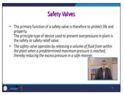
The primary function of a safety valve is to protect life and property. As discussed in the previous example, a domestic pressure cooker is equipped with two different types of safety
