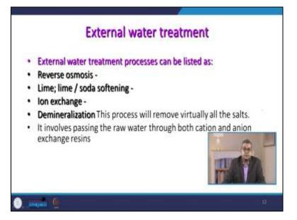
We need to have some external water treatment protocols because there are various sources of water may be the natural water may be surface water may be groundwater may be the, subsurface water, maybe you are taking water from the river or a canal or maybe municipal water. So, you cannot feed this water directly to the boiler because there are certain inherent impurities.
