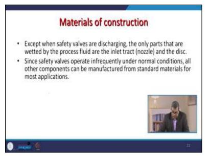
Sometimes people ask about the material of construction of these safety valves except when the safety valve is discharging. The only part that is wetted by the process fluid is the inlet tract or nozzle and the disc. And usually, the disc and seats are directly in touch with the working fluid.
