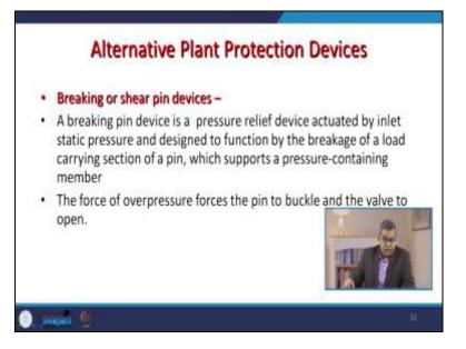
Sometimes the breaking or shear pin devices are also being used. Usually a breaking pin device is a pressure relief device actuated by inlet static pressure and designed to function by the breakage of a load carrying section of a pin that supports a pressure-containing member. The force of overpressure forces the pin to buckle out and the valve to open. The valve can then be reseated after pressure is removed and a new pin need to be installed over there.
