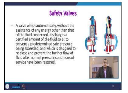
Usually when we; talk about safety devices, a valve automatically, without the assistance of any energy other than that, the fluid in question discharges a certified amount of fluid. So, as to prevent a predetermined safe pressure from being exceeded and which is designed to reclose and prevent the further flow of fluid after normal pressure conditions of the service have been restored. These are the two essentials of safety valves.
