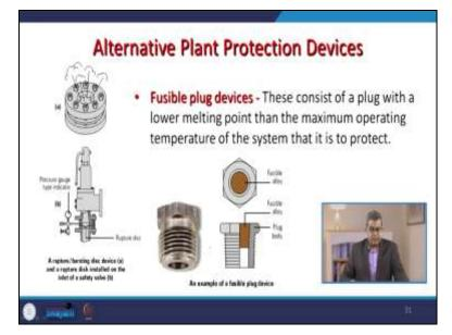
Here you see the fusible plug device or a safety device like your domestic pressure cooker. Here you see these consist of a plug with a lower melting point than the maximum operating temperature of the system that is protected. So, basically, it is meant as a temperature protection device. This is a simple example you can screw it. This is the plug body, and this is the fusible alloy sometimes elastomers are also being used.
