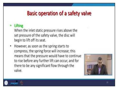
Let us talk about some basic operations of a safety valve, and the foremost operation is called lifting. When the inlet static pressure rises above the safety's set pressure, the disc will begin to lift off the seat. as soon as the spring starts to compress as you we discussed in this particular figure the spring force will increase, and this means that pressure would have to continue to rise before any further lift can occur and for there to be any significant flow through the valve.
