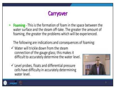
The second aspect is foaming. This is the formation of foam in the space between the water surface and the steam takeoff. The greater the amount of foaming, the greater the problems which can be experienced. There are certain indications and consequences of foaming. One is that water will trickle down from the gauge glass's steam connection, which makes it difficult to accurately determine the water level.
