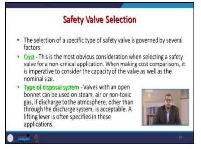
Another thing is that the type of disposal system valve with an open bonnet can be used on steam air or nontoxic gas but is acceptable if discharged to the atmosphere other than through the discharge system. A lifting lever is often specified in these applications, as you see in the figure. (Refer Slide Time: 19:45)
