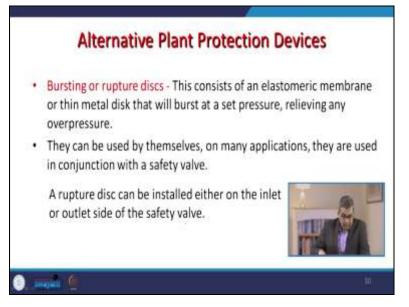
We were talking about the bursting or a ruptured disc. This consists of an elastomeric membrane or thin metal disc that will burst at a set pressure-relieving any overpressure. Sometimes it also gives an edge towards the high-temperature system. If the melting point of these elastomeric membranes or disc operating temperature is more than the melting point of these elastomeric membranes may meltdown to release the excessive pressure as well as the temperature.
