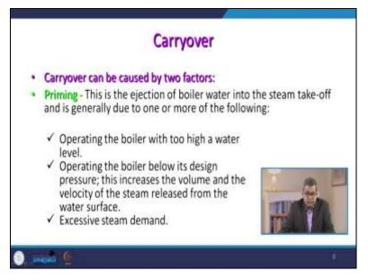
Let us talk about the carryover. Two factors can cause this carryover. One is the priming. This is the ejection of boiler water into the steam takeoff and is generally due to one may be one or more reasons attributed to this one operating the boiler with the too high water level. So, again it is very dangerous because you are imparting an excess amount of energy to produce the steam. Operating the boiler below the design pressure
