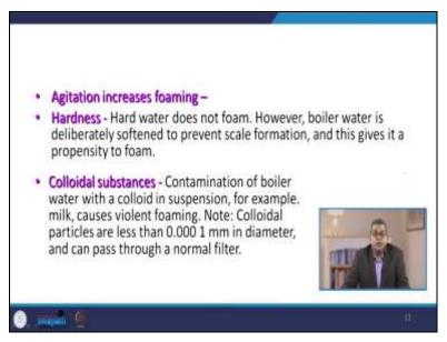
Sometimes colloidal substances are also very important. The contamination of boiler water with the collides in suspension. For example, milk causes violent foaming. Collider particles are those that are less than 0.0001 millimeters in diameter and can pass through a normal filter. So, all these need to be addressed. We have already discussed this TDS concept.
