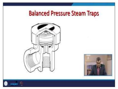
This is the balanced pressure steam trap here, and some weighted discs are there if there is a change in density. So, it may open or close just to facilitate the passage of condensate.
