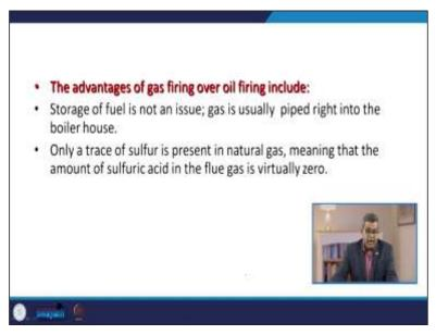
Advantages of gas firing over oil firing because we; discussed that oil is a bit superior to coal. Similarly, the gas firing has more advantages compared to the oil firing. This includes that the storage of fuel is not an issue. Gas is usually piped right into the boiler house. Only traces of sulphur are present in natural gas, meaning that the amount of sulfuric acid in the flue gases is minimal. Another choice of fuel is waste, waste as a primary fuel.
