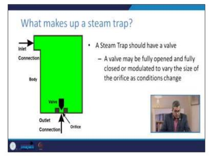
A steam trap should have a valve. A wall may be fully opened or fully closed, or modulated to vary the size of the orifice as per the condition changes. Here you see that this is the valve, and it changes as per the prevailing conditions. a stream trap should have an operator. This operator usually senses when to move the wall and supplies the power to move the wall. Traps are different in the type of wall and types of operator use.
