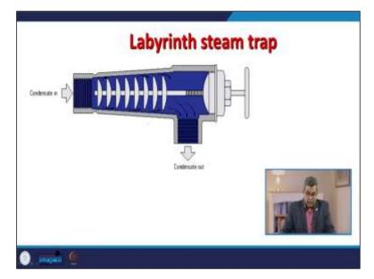
Again, you see that the labyrinth type of steam trap is very common and very useful. Here these discs are attached in a graduating reducing manner, and this is the crown wheel through which you can adjust the length of these discs; and by this way, this not only imparts a hindrance to the passage. So, any kind of esteem may get condensed over time, which can allow the safe passage for the condensate out.
