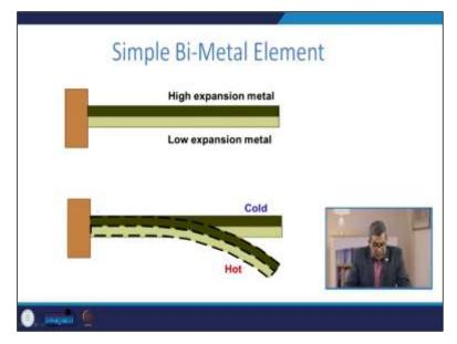
When we talk about this simple bi-metal element, two metals with different expansion aspects are infused together. Here you see that this is the high metal, the high expansion metal, and here the other infused metal is the low expansion metal. So, when any temperature change occurs, there may be slight deformation in these rods or in these operators, which can reduce the flow or change or alter the flow, and the steam trap works.
