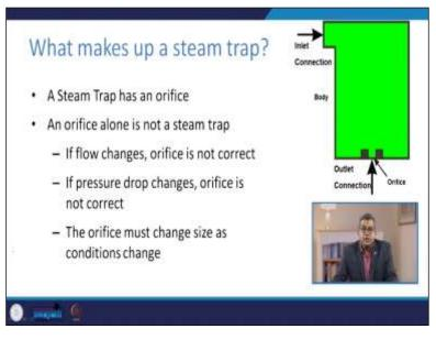
The question is, again, what makes up a steam trap. Usually, a steam trap has an orifice you can see over here, and an orifice alone is not a steam trap. If flow changes orifice is not correct if pressure drop changes or if it is not correct, if the orifice must change size as conditions changes, that is the thing. Here you can see the inlet connection, body, and outlet connection. All these are some of the rough diagrams of the steam trap.
