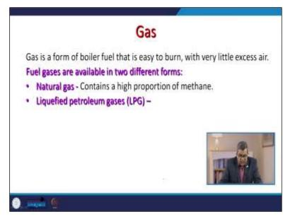
Another choice is the gas. Gas is a form of boiler fuel that is easy to burn with very little excess air. Fuel gases are available in two different forms: natural gas containing a high proportion of methane, almost 85 to 90%, and LPG, the liquefied petroleum gas.
