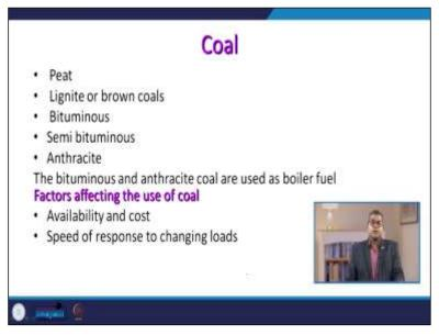
Let us briefly talk about coal. There are different types of coals in practice peat lignite or brown coal, bituminous, semi bituminous anthracite. The bituminous and anthracite coals are used for the boiler fuel. When we are using these types of fuels, there are several factors affecting the use of
