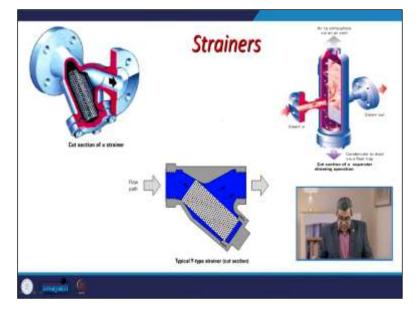
These are some of the examples of the strainers cut section of the strainer. Here it is a more pictorial view here, the steam is coming inside, and it strikes the plate that is the perforated plate, and because of the striking, some of the steam may get condensed. So, you can remove the system, and the purest form, purified, or restrained form of steam is coming out. This is the inner anatomy of the strainer. This is a flow path you can see that this is the strainer.
