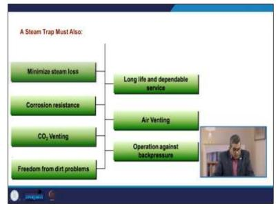
So, a steam trap must also minimize steam loss, which is again very important. It must be corrosion resistant, impart carbon dioxide venting, and impart freedom from dirt problems. All these things are essential for the long life and dependable service of the boiler steam piping network etc. Apart from this, the steam trap must also provide air venting. It must provide operation against the backpressure.
