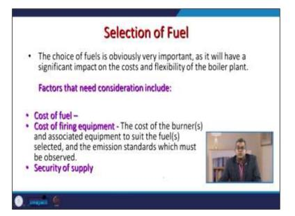
The cost of firing equipment, the cost of burners, and associated equipment to suit the fuels selected and emission is standard which must be observed. Then the security of supply sometimes the disturbance may create the problem and thereby it may adversely impact to the operation of your boiler house.
