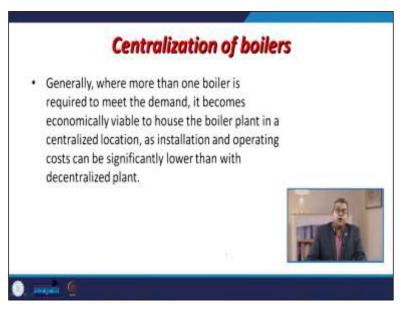
Installation and operating costs can be significantly lower than with the; decentralized plant. Centralization offers various benefits over the use of this dispersed smaller boiler that, is more choices of fuel and tariff.
