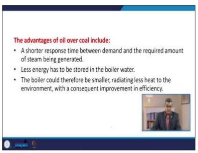
When we have the choice between oil and coal, there are certain advantages associated with oil over coal, including the shorter response time between the demand and the required amount of steam being generated. Less energy has to be stored in the boiler water because of this shorter
