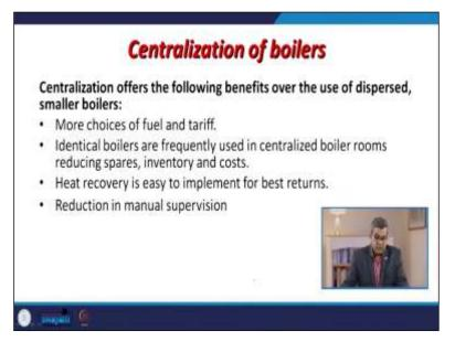
Identical boilers are frequently used in the centralized boiler rooms, reducing the inventories cost and spare cost. Heat recovery is quite easy to implement for the best return and the reduction in manual supervision. Economic size and the sizing of the boiler plant to suit the diversification in demand sometimes with the centralization of the boiler exhaust emissions are easily monitored and controlled. You may have only one stake through which you can discharge the things.
