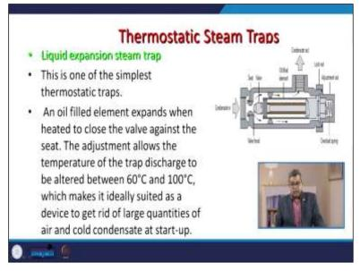
There are some thermostatic steam traps in which the liquid expansion steam trap usually is one of the simplest forms of the thermostatic trap. An oil-filled element usually expands when heated to close the wall against the seed. The adjustment allows the temperature of the trap discharge to
