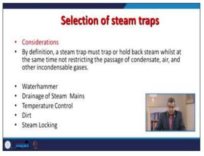
We discussed a lot of different types of steam traps. The question arises of how we can go for a proper steam trap. This is one of the fundamental questions. So, while selecting the proper steam trap, there must be certain considerations, and by definition, a steam trap must trap or hold back
