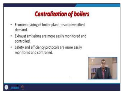
Similarly, these protocols' safety and efficiency are more easily monitored and controlled because it is centrally located. See when sometimes the fuel for the boiler is a very debatable aspect because it has a various parameters to be addressed. Usually, there are three most common types of fuels used, coal, oil, and gas. Industrial or commercial waste is sometimes used in certain boilers and the electricity for electrode boilers.
