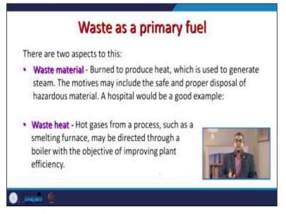
One example is hospital waste; another is the waste heat hot gases from a process like the exothermic process in a chemical reaction. Another is the smelting furnace, which may be directed through a boiler to improvise the plant efficiency. So, we discussed the different types or choices of fuel. The question arises: What should be the phenomena through which we can select the appropriate fuel.
