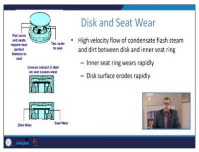
High velocity the flow of condensate to flash stream and dirt between the disc and inner seat rings sometimes it can create a problem and this inner seat this one inner seat ring wears rapidly, and disc surface erodes rapidly.
