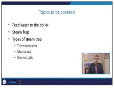
In the previous lecture, we discussed the feed water quality feed water supply of the boiler. This chapter will discuss the remaining part of this feed water supply or quality or the importance of feed water to the boiler. We will discuss the steam traps, especially regarding the different types attributed to the thermodynamic steam trap mechanical thermostatic steam traps.
