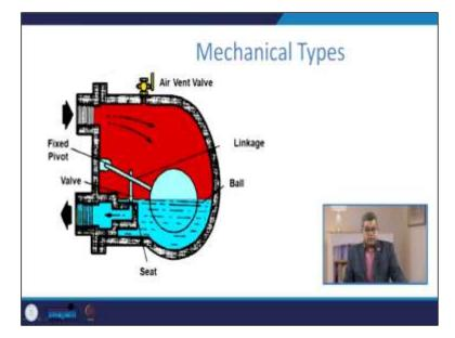
There are certain mechanical traps here you see that this is a float ball or float valve. It is closely linked with the fixed pivot, and it is attributed to the valve, and this is the air vent wall. So, if this particular, I mean the level of water goes up in the in this steam trap, then automatically this wall opens to facilitate the drainage of condensate water and to facilitate the steam entrapment.
