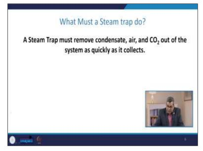
The steam trap must remove condensate air or any kind of co to interrupt from the system as quickly as it collects. There should be no term, and theoretically, there should not be any retention time.
