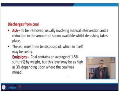
Emission usually coal contains 1.5% of sulfur by weight, but this level may be high as 3% depending upon where the coal was mined, and trust me, this creates a huge problem with respect to the environmental aspect.
