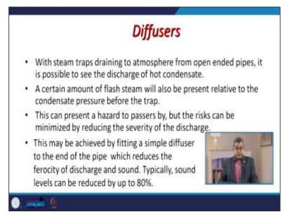
Apart from these accessories, there are certain diffusers are being used in the steam line or steam traps. With the steam trap draining into the atmosphere from an open-ended pipe, it is possible to see the discharge of hot condensate. A certain amount of flash steam will also be present relative to the condensate pressure before the trap. This can present a hazard to a passerby, but the risk can be minimized by reducing the severity of the discharge.
