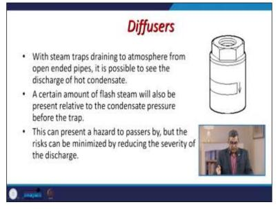
This is the typical diffuser. With the steam trap draining into the atmosphere from an open-ended pipe, it is possible to see the discharge of hot condensate. A certain amount of flash steam will also be present relative to the condensate pressure before the trap. This can be this can present a hazard to the passerby, but the risk can be minimized by reducing the severity of the discharge.
