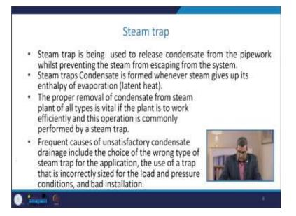
The steam traps are being used to release the condensate from the pipework while preventing the steam from escaping into the system. Steam trap condensate usually, when the condensate is formed, the steam gives up its enthalpy of evaporation called the latent heat. The proper condensate removal from the steam plant of all types is vital. If we; need to work the plant efficiently and the steam trap commonly performs this operation.
