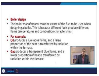
This is because a different fuel produces a different type of flame temperature and combustion characteristics. For example, oil produces luminous flame, and the radiation transfers a large proportion of the heat within the furnace. Gas produces the transparent blue flame, and the radiation transfers a lower proportion of heat within the furnace. So, in this particular lecture, we discussed the various accessories attributed to steam generation, especially the boilers.
