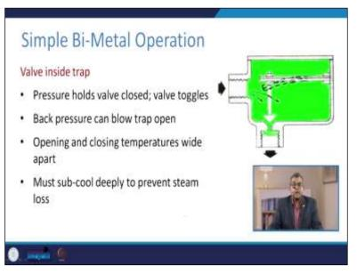
You can see this is a more pictorial thing. Here you see that when this metal deforms, it usually closes this wall. So, it restricts the passage of either steam or water. Usually, this valve is operated through this bimetallic strip. Usually, the wall inside trap pressure holds the valve closed—this
