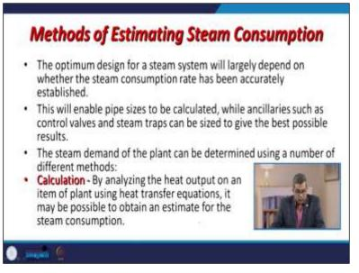
Another important point in the steam generation unit is estimating steam consumption. The optimum design for a steam system largely depends on whether the steam consumption rate has
