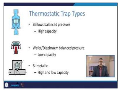
So, the thermostatic trap system is foremost when we talk about the different types of traps. Here this is again a different type of trap like bellows balance pressure are having a very high capacity like this then wafer diaphragm balanced pressure slightly lower capacity. Here you see that there are certain bimetallic types of thermostatic traps with high and low capacity in the wafer and the diaphragm. So, these are the biometrics we will discuss in due course of time.
