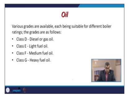
The next fuel is oil. Usually it is graded based on the requirement based on various refiners etc. So, various grades are available and suitable for different types of a boilers rating and these grades are like class D diesel or gas oil class C light fuel oil class F medium fuel wire class G heavy fuel oils, etc.
