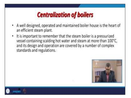
See, when we talk about the boiler and these accessories in a mounting, another concept is usually coming to the picture: the centralization of the boiler. Sometimes it is very catchy or a buzzword. The reason is that if we are having the centralization of the boilers concept, then we may have the facility to have one steam distribution network, but simultaneously it offers a variety of disadvantages related to the varying load.
