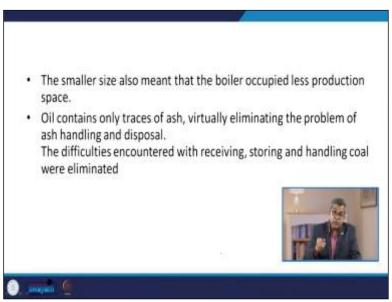
The oil contains only traces of ash and virtually eliminates the ash handling and disposal problem, which is a very burning problem. The difficulty is encountered while receiving, storing and handling coal usually it is being eliminated.
