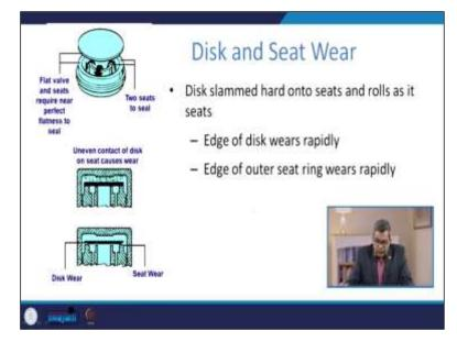
Other types of steam traps are disc and seat types of systems. Here you see that this is the disc that is usually seated over here. This is the two-seat seat to seal, and this is the flat wall and seats required near perfect to the flatness of seal. So, this is the usual condition, and if any kind of deformation occurs, this may open, and the water or steam whatever can come out.
