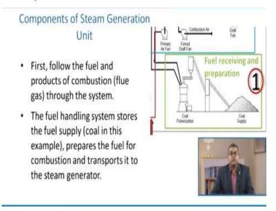
So, let us take them one by one. Because if you follow the fuel and a product of combustion through the system, the fuel handling system usually stores the fuel supply that is cool for this particular example. This prepared the fuel for combustion and transported it to steam generation as you know that we require some specific size in terms of coal.
