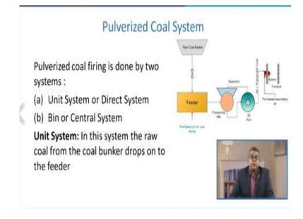
Now let us talk about the pulverized coal system. We have already discussed the concept of polarization in the previous lectures. So, pulverized coal firing is usually done by two systems, one is the direct system or called a unit system, and the second is the central system or bin type. The raw coal from the coal bunker drops into the feeder in the unit system. That is the raw coal bunker, and it is a feeder. And then this is a polarizing mill, and through this, it goes to the desired station.
