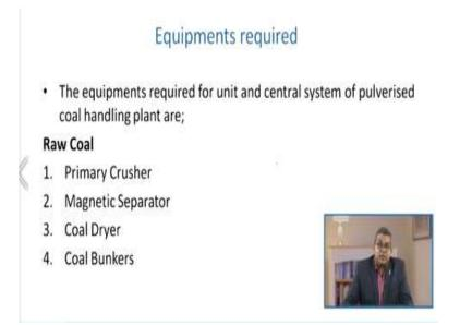
You require the primary crusher for raw coal because it usually forms in a big lump. Then magnetic separators because some metal, especially iron impurities, can be removed a priory. You must have a coal dryer; we have already discussed that it contains a significant quantity of water and moisture. So, before it goes to either pulverization or furnace, it should be dried and must require the coal bunkers.
