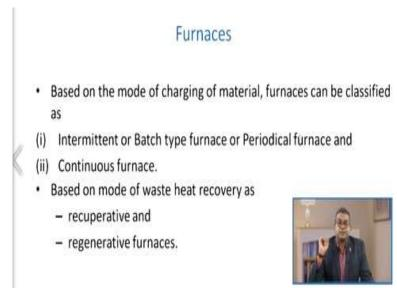
Another classification may be based on the mode of charging of material. These furnaces can be classified into intermittent or batch-type furnaces or periodical and continuous furnaces. Sometimes based on the mode of waste heat recovery, one is recuperative, and the second one is the regenerative furnace.
