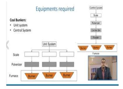
Now here you see the coal bunkers both for the unit and central systems. Now here is your unit system. It would help if you had the scale then the different pulverization units, and it goes to the burner, and you may have different burners. Here in the central system, you must have a scale, then perform the pulverization operation goes to central bin, feeder, and through the feeder, it goes to the different furnaces through the burner.
