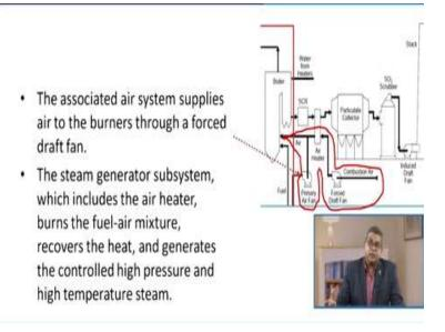
So, you can go for, say, polarization, grinding, etc., whatever is required for this one that is attributed to the fuel receiving and preparation section. When you have selected the fuel, you have dressed the fuel as per the requirement, and then the next aspect is the combustion air. Because it is a combustion reaction, you need to supply the air by utilizing the fact that it contains 21% of oxygen.
