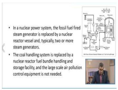
In the nuclear power system, the fossil fuel fired steam generator is replaced by the nuclear reactor vessel, typically two or more steam generators. This is what you can say about the supplement thing in the nucleophile reactors. The coal handling system is replaced by the nuclear reactor fuel bundle handling and storage facilities, and the large-scale pollution control equipment is not needed.
