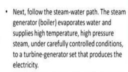
The steam may also be reheated in the steam generator, after passing through part of a multistage turbine system, by running the exhaust steam back to the boiler convection pass
