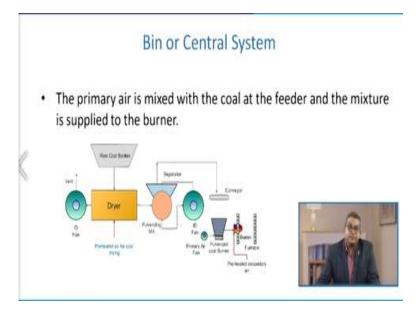
Now here you see that this is the raw coal bunker dryer, which is the pulverizing mill, and to this, it is conveyed to the desired station. And here you see that we have the primary fan, and this pulverized coal burner is subjected to the furnace. Now here you are mixing the primary air in the system to have combustion properly.
