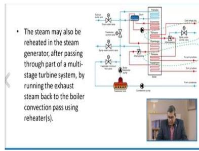
Apart from this, you may utilize whatever condensate is being formed as a source of feed water because sometimes this condensate is available at a substantially high temperature. So, it always enhances the boiler efficiency if we use it. Now see, when we talk about the steam, this may also be reheated in the steam generator. And if we pass through the multiple-stage turbine system, we can extract the work.
