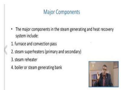
Now let us talk about the major components. The major components in the steam-generating and heat recovery system they are including furnace and convection pass, super steam heaters may be primary and secondary, steam reheaters boiler, or steam-generating banks.
